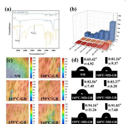
Fig. 4 (a) Infrared spectra of MD-HBP-NH<sub>2</sub> after reaction. (b) Surface roughness measurement results (Sa, Sz and Sq). (c) Surface 3D topography of the samples. (d) The initial water contact angle and the water contact angle after five seconds.
