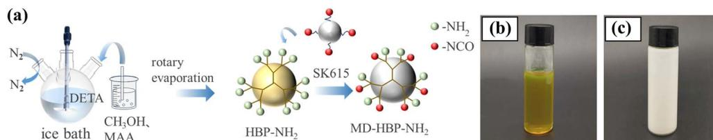
Fig. 1 (a) Synthetic pathways for HBP-NH<sub>2</sub> and MD-HBP-NH<sub>2</sub>. (b) HBP-NH<sub>2</sub>. (c) MD-HBP-NH<sub>2</sub>.
