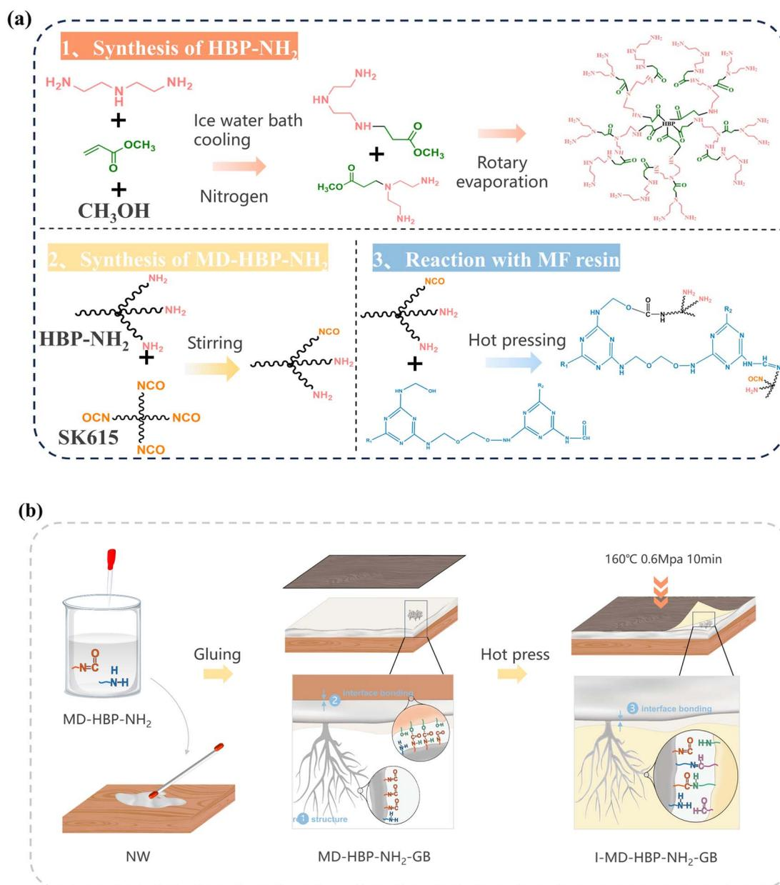
Fig. 2 (a) Synthesis and reaction process of MD-HBP-NH<sub>2</sub>. (b) The preparation procedure for a wood/impregnated grafted blockboard sample (I-MD-HBP-NH<sub>2</sub>-GB).
