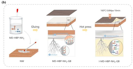
Fig. 2 (a) Synthesis and reaction process of MD-HBP-NH<sub>2</sub>. (b) The preparation procedure for a wood/impregnated grafted blockboard sample  $(I-MD-HBP-NH_2-GB)$ .
