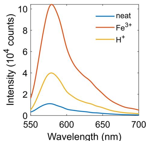
Fig. 2 Fluorescence spectra excited at 510 nm for 1 mg mL<sup>-1</sup> aqueous suspensions of RBA@SiNCs: as prepared (blue curve) and after a 1 month exposure to 5 mM Fe<sup>3+</sup> (red curve) or H<sup>+</sup> (yellow curve). As Fe<sup>3+</sup> ions exhibit strong light absorption in the visible range, they were removed by washing RBA@SiNCs with centrifugation before acquiring the spectrum.
