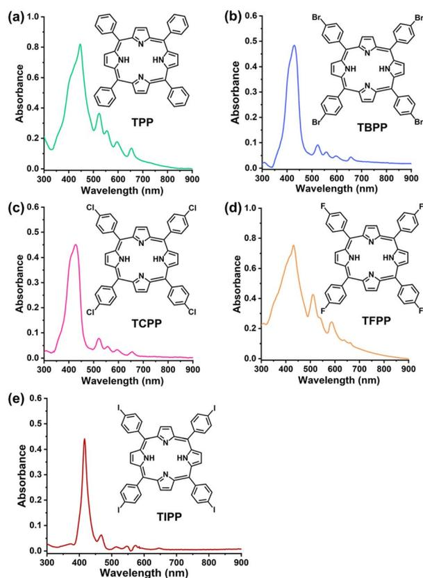
Fig. 1 (a–e) Chemical structures and UV-Vis spectra of TPP, TBPP, TCPP, TFPP, TIPP (20  $\mu\text{M}$ ) in PBS. TPP, 5,10,15,20-tetraphenyl porphyrin. TBPP, 5,10,15,20-tetrakis(4-bromophenyl)porphyrin. TCPP, 5,10,15,20-tetrakis(4-chlorophenyl)porphyrin. TFPP, 5,10,15,20-tetrakis(4-fluorophenyl)porphyrin. TIPP, 5,10,15,20-tetrakis(4-iodophenyl) porphyrin.
