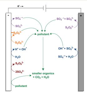
Fig. 2 Electrochemically activated persulfate.
