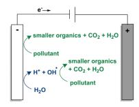
Fig. 1 Anodic oxidation.
