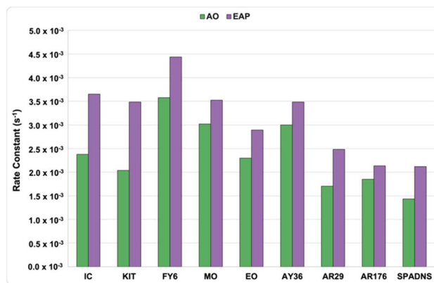
Fig. 6 First order rate constants of nine dyes under AO and EAP conditions.
