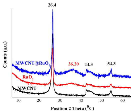
Fig. 3 XRD spectra of MWCNT and MWCNT@RuO<sub>2</sub>.
