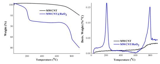
Fig. 5 TGA and DTG curves of MWCNT and MWCNT@RuO<sub>2</sub>.
