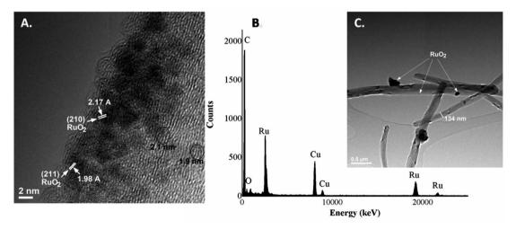
Fig. 2 (A) HRTEM images, (B) TEM images and (C) EDX spectra of MWCNT@RuO<sub>2</sub>.
