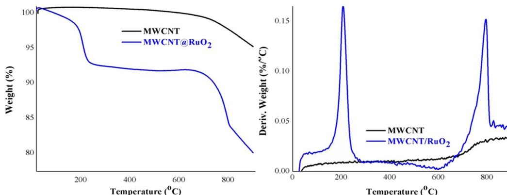
Fig. 5 TGA and DTG curves of MWCNT and MWCNT@RuO<sub>2</sub>.
