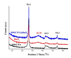
Fig. 3 XRD spectra of MWCNT and MWCNT@RuO<sub>2</sub>.
