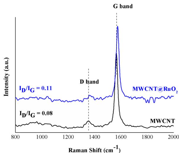
Fig. 4 Raman spectra of MWCNT and MWCNT@RuO<sub>2</sub>.
