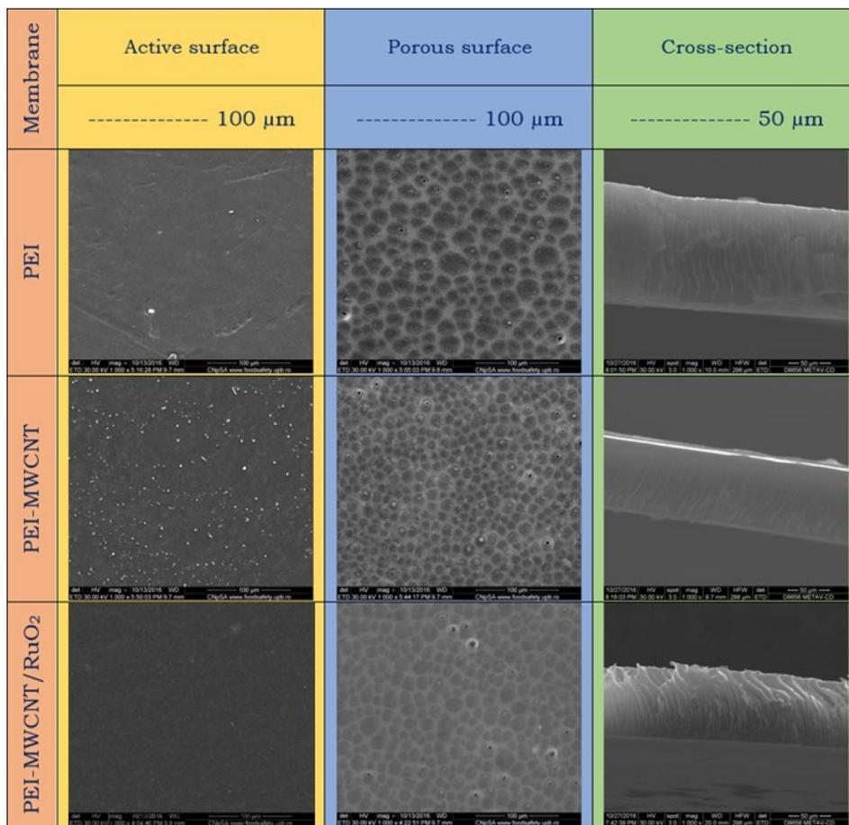
Fig. 8 SEM images of the PEI and composite membranes.
