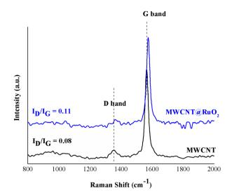
Fig. 4 Raman spectra of MWCNT and MWCNT@RuO2.
