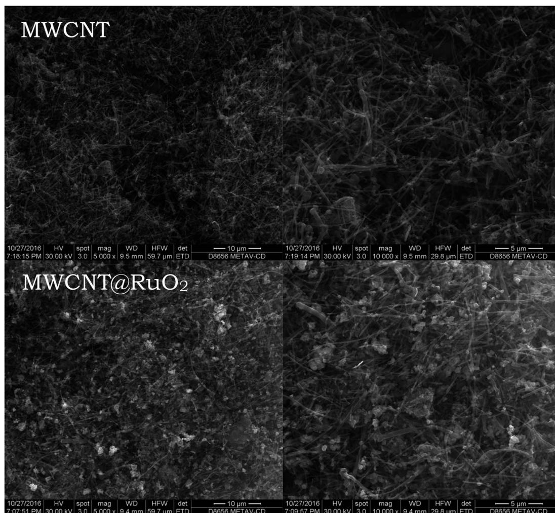
Fig. 1 SEM images of the MWCNT and MWCNT@RuO<sub>2</sub>.
