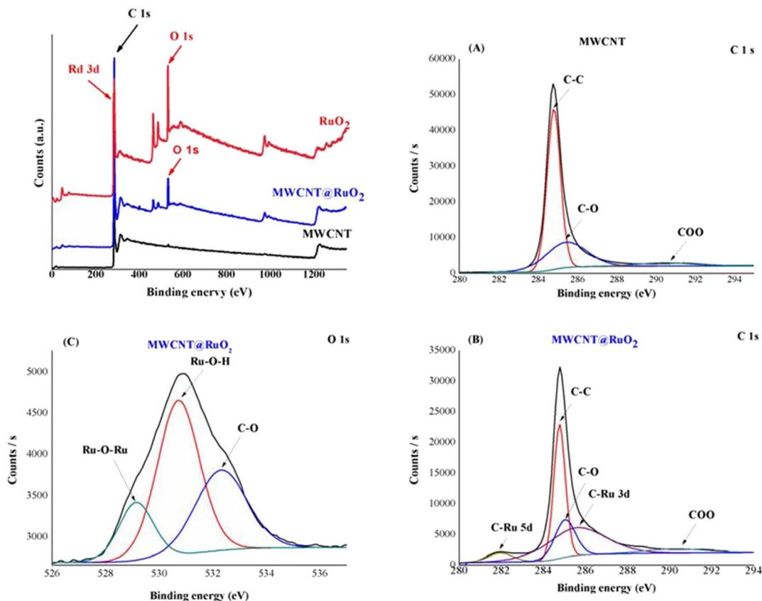
Fig. 6 XPS survey spectra of MWCNTs before and after decoration with  $\text{RuO}_2$ : high-resolution C 1s spectra of MWCNT (A) and MWCNT@ $\text{RuO}_2$  (B); and high-resolution O 1s spectra of MWCNT@ $\text{RuO}_2$  (C).
