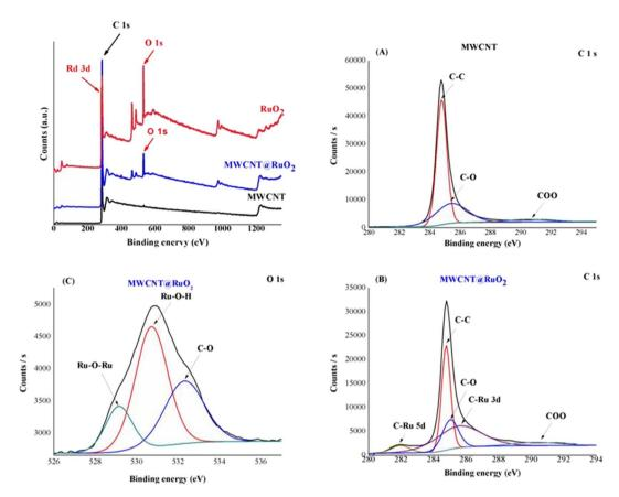
Fig. 6 XPS survey spectra of MWCNTs before and after decoration with RuO<sub>2</sub>: high-resolution C 1s spectra of MWCNT (A) and MWCNT@RuO<sub>2</sub> (B); and high-resolution O 1s spectra of MWCNT@RuO<sub>2</sub> (C).
