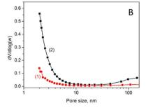
Fig. 2 N<sub>2</sub> adsorption-desorption isotherms at liquid nitrogen temperature (A) and pore size distribution curves (B) for the nonactivated (1) and the activated (2) luffa biochar
