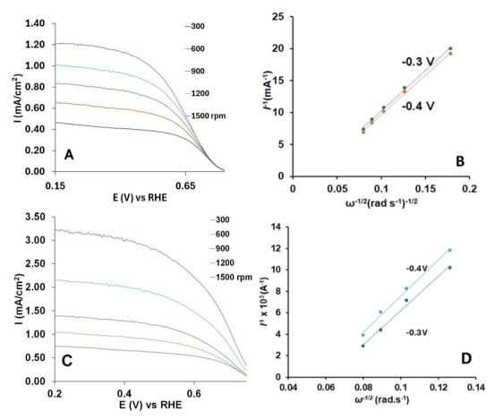
Fig. 6 Non-activated (A and B) and activated (C and D) luffa biochar: (A and C) rotating disk electrode voltammetry curves of  $O_2$  reduction in an aqueous solution of 0.1 M KOH and various rotation rates; (B and D) corresponding Koutecky–Levich plots at -0.3 and -0.4 V vs. NHE. Scan rate: 25 mV s<sup>-1</sup>.
