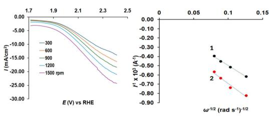
Fig. 8 Rotating disk electrode voltammetry curves for OER in an aqueous solution of 0.1 M KOH at various rotation rates for non-activated luffa biochar electrode and Koutecky-Levich plots of non-activated (1) and activated (2) luffa biochar at 1.6 V vs. NHE. Scan rate: 25 mV s<sup>-1</sup>.
