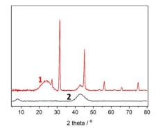
Fig. 3 XRD patterns of the non-activated (1) and the activated (2) luffa biochar.
