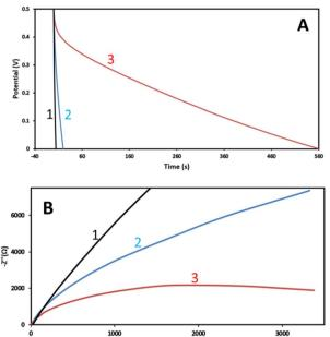
Fig. 5 (A) Galvanostatic discharge curves of biochar-electrode symmetric cells for measuring specific capacitance. The flowing current was: 10  $\mu$ A, CB/CC (1); 200  $\mu$ A, non-activated biochar/CC (2); and 200  $\mu$ A, activated biochar/CC (3). (B) Impedance curves for CB (1); non-activated (2) and activated (3) biochar electrodes. The electrolyte was in all cases 0.5 M aqueous KOH.
