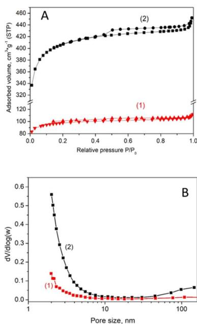
**Fig. 2** N<sub>2</sub> adsorption-desorption isotherms at liquid nitrogen temperature (A) and pore size distribution curves (B) for the non-activated (1) and the activated (2) luffa biochar.
