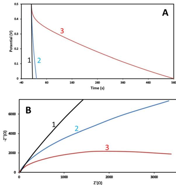
Fig. 5 (A) Galvanostatic discharge curves of biochar-electrode symmetric cells for measuring specific capacitance. The flowing current was: 10  $\mu\text{A}$ , CB/CC (1); 200  $\mu\text{A}$ , non-activated biochar/CC (2); and 200  $\mu\text{A}$ , activated biochar/CC (3). (B) Impedance curves for CB (1); non-activated (2) and activated (3) biochar electrodes. The electrolyte was in all cases 0.5 M aqueous KOH.
