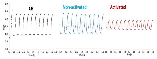
Fig. 10 Charge-discharge cycles for rechargeable Zn-air batteries made by using CB, non-activated and activated luffa biochar as electrocatalysts on the air-electrode.
