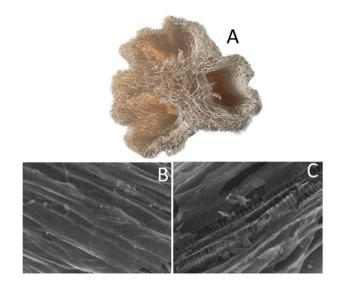
Fig. 1 A picture of the original luffa (A); and SEM images of non-activated (B) and activated (C) luffa biochar. The scale bar for SEM is 50  $\mu$ m.
