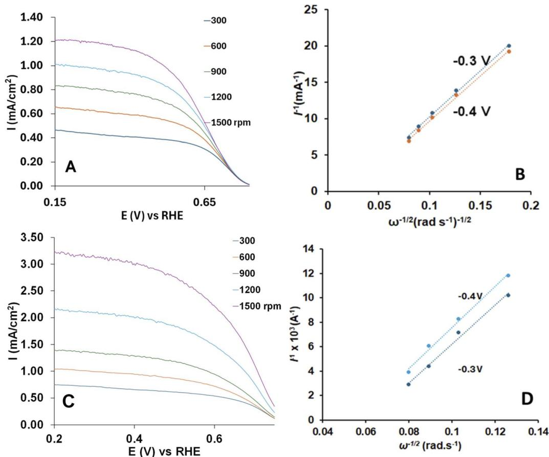
Fig. 6 Non-activated (A and B) and activated (C and D) luffa biochar: (A and C) rotating disk electrode voltammetry curves of O<sub>2</sub> reduction in an aqueous solution of 0.1 M KOH and various rotation rates; (B and D) corresponding Koutecky–Levich plots at -0.3 and -0.4 V vs. NHE. Scan rate: 25 mV s<sup>-1</sup>.
