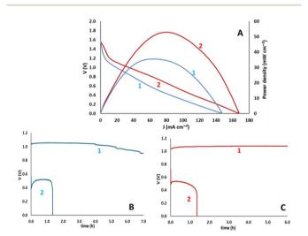
Fig. 9 (A) Linear sweep voltametry data for two Zn-air batteries made with non-activated (1) and activated (2) luffa biochar electrocatalyst. (B) Galvanostatic discharge behavior of a battery made with non-activated biochar at 20 mA (1) and 100 mA (2). (C) Corresponding data for activated biochar.
