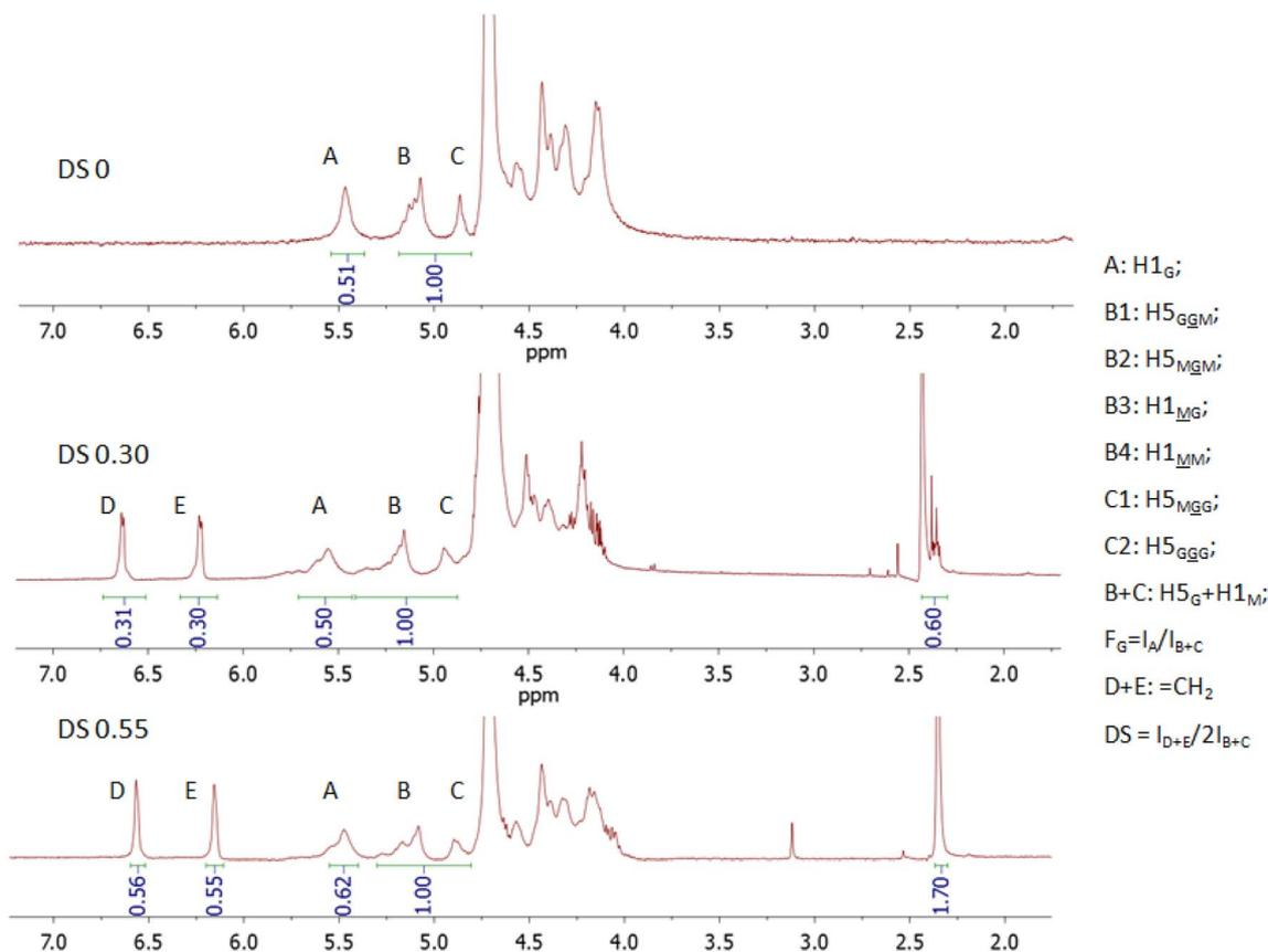
Fig. 1 <sup>1</sup>H NMR spectra of ALG and M-ALGs.
