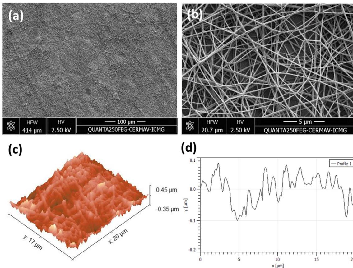
Fig. 6 (a) Broad and (b) enlarged SEM images, AFM (c) 3D topographical image and (d) 2D surface roughness profile of the needle electrospun M-ALG fiber mat (DS 0.55).
