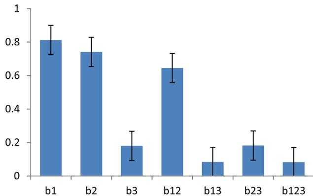
Fig. 4 Normalized coefficients of  $2^3$  factorial design for the relationship between the concentrations of the solution components (b1: ALG concentration, b2: PEO concentration, b3: Triton X-100 concentration) and viscosity.
