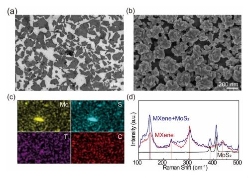
Fig. 2 Morphology and structural analysis of the MXene/MoS<sub>2</sub>. SEM image of (a) the LB-MXene nanosheets onto a  $SiO_2/Si$  substrate, (b) the synthesized MoS<sub>2</sub> on LB-MXene, (c) EDS mapping images of MXene/MoS<sub>2</sub>, (d) Raman spectrum of MoS<sub>2</sub>, MXene, and MXene/MoS<sub>2</sub>.
