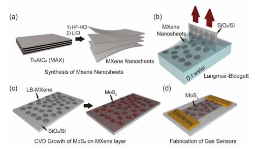
Fig. 1 Schematic illustration of the synthesis of MXene/MoS<sub>2</sub>. (a) Preparation of MXene nanosheets from MAX phase, (b) thin layer formation of MXene on  $SiO_2/Si$  substrate using LB technique. (c) Growth of MoS<sub>2</sub> on LB-MXene, and (d) fabrication of LB-MXene/MoS<sub>2</sub> based gas sensor.
