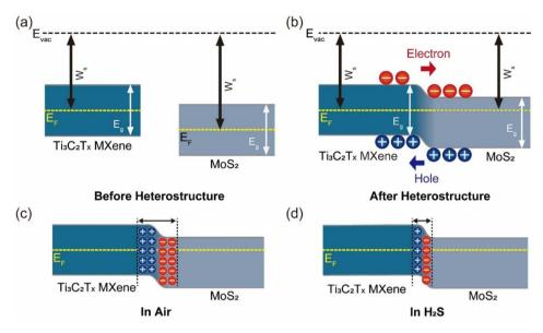
Fig. 4 Band diagram of chemi-resistive gas sensor based on MXene/MoS<sub>2</sub> layer. Band diagrams before (a) and after (b) forming the heterostructure between MXene and MoS<sub>2</sub>. Band diagram under air (c) and  $H_2S$  (d) injection.
