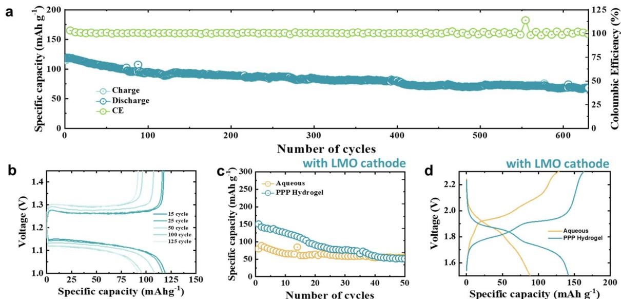
Fig. 7 (a) Long cycling performance and (b) galvanostatic charge/discharge curves of PPP hydrogel-based Zn||LFP hybrid pouch cell battery at 0.1C. (c) Discharge capacity and (d) voltage/capacity curves of the PPP hydrogel and aqueous electrolyte-based Zn||LiMn<sub>2</sub>O<sub>4</sub> hybrid pouch cell batteries.
