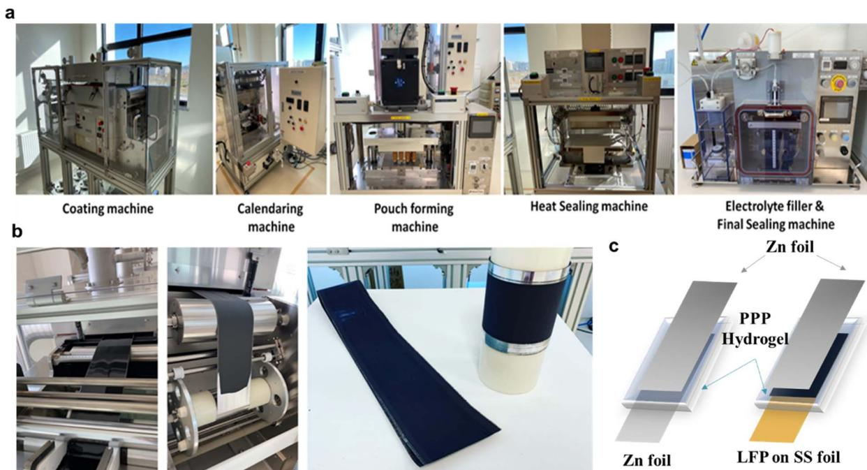
Fig. 4 (a) The pilot line for pouch cell preparation. (b) Preparation of the cathode. (c) Schematic illustration of the symmetric Zn||Zn (left) and full Zn||LiFePO<sub>4</sub> (right) pouch cell assembly.
