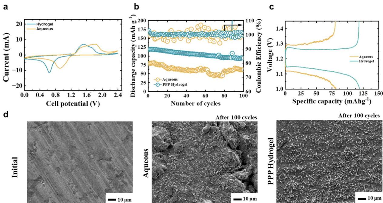
Fig. 6 (a) CV of the PPP hydrogel and aqueous electrolyte-based full Zn||LFP pouch cells at  $0.1 \text{ mV s}^{-1}$ . (b) Discharge capacity and coulombic efficiency, and (c) charge–discharge curve comparison PPP hydrogel and aqueous electrolyte-based hybrid Zn||LFP pouch cell battery system tested. (d) SEM images of the Zn anode surface after 100 charge–discharge cycles.
