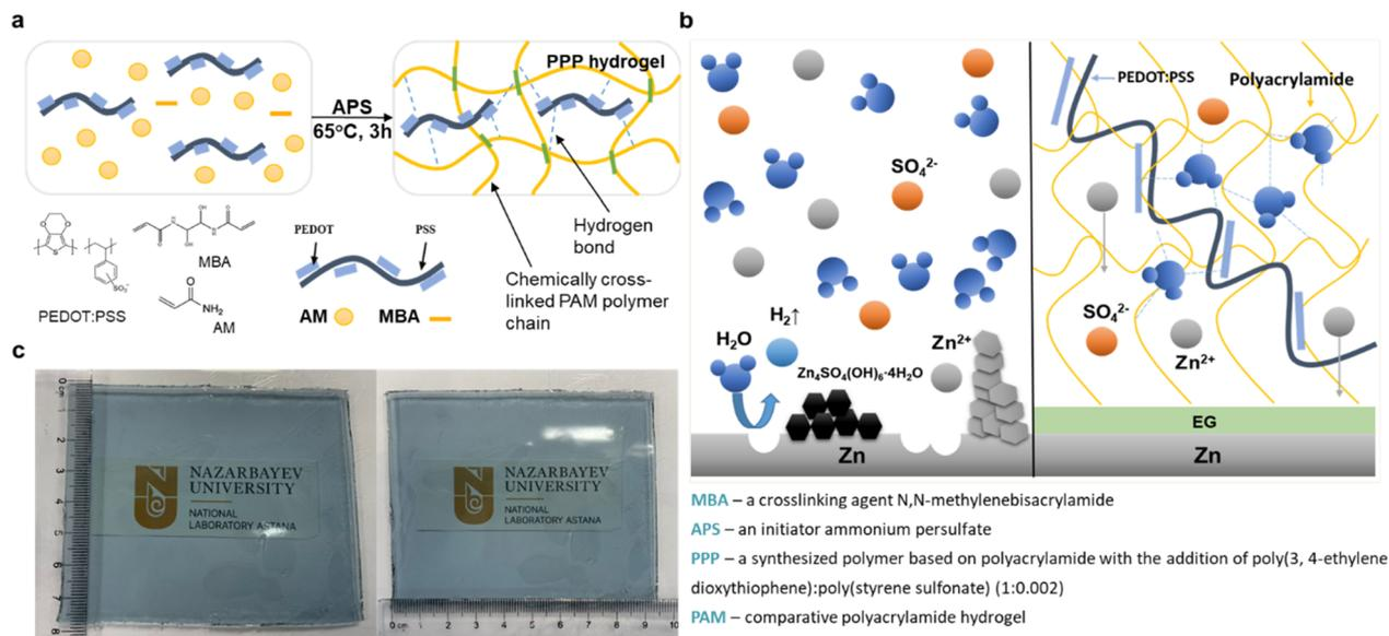
**Fig. 1** (a) Schematic illustration of the one-pot PPP hydrogel polymerization and chemical and physical cross-link formation. (b) Schematic of the hydrogel electrolyte with an ethylene glycol additive working principle preventing side reactions and modulating water activity. (c) Photos of prepared PPP hydrogel.
