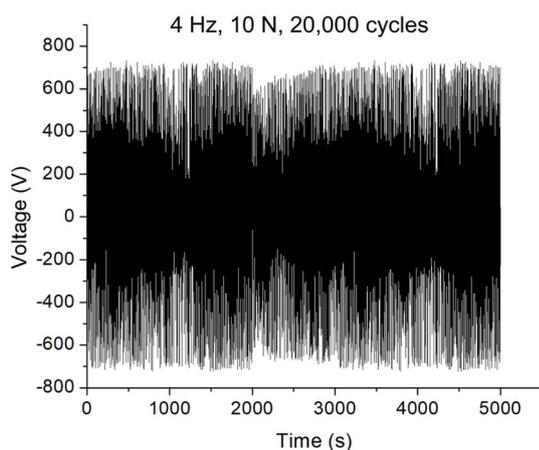
Fig. 9 Long-term cycling test of TENGs (operating conditions: 4 Hz, 10 N, 20 000 cycles).
