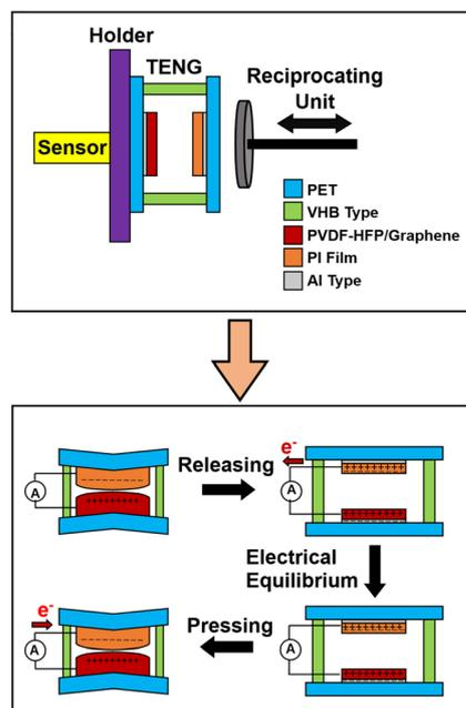
Fig. 1 Schematically the working mechanism of lab-made TENGs.
