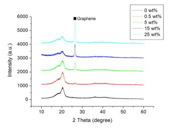
Fig. 4 XRD patterns of the PVDF-HFP nanofibers filled with different percentages of graphene.
