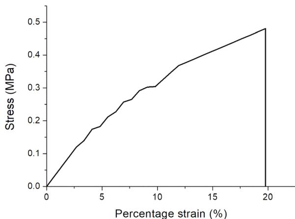
Fig. 3 Stress–strain curve of the 15% graphene-filled PVDF-HFP nanofibers.
