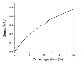
Fig. 3 Stress-strain curve of the 15% graphene-filled PVDF-HFP nanofibers.
