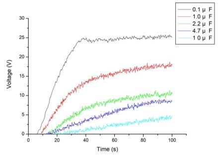
Fig. 12 The voltage curves recorded while charging capacitors with various capacitances (0.1, 1, 2.2, 4.7 and 10 μF) using the graphene/PVDF-HFP TENGs.
