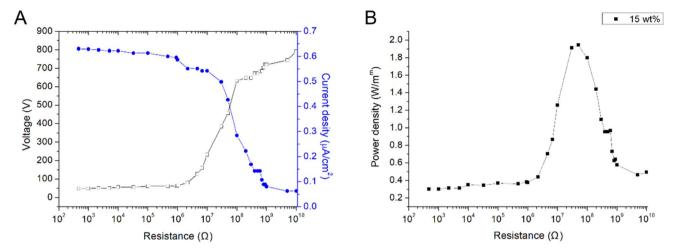
Fig. 8 (A) Output voltage and current density, and (B) power density of TENGs composed of different-weight-percentage graphene filled PVDF-HEP nanofibers
