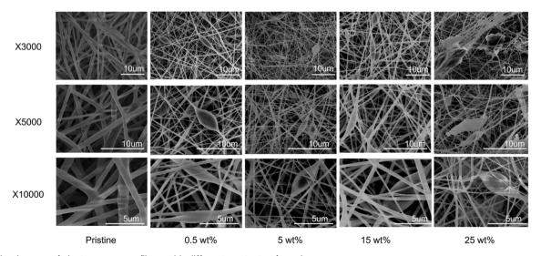
Fig. 2 Microimages of electrospun nanofibers with different contents of graphene.
