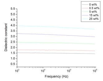
Fig. 5 Frequency-dependence of the dielectric constant of graphene/ PVDF-HFP nanofibrous mats.
