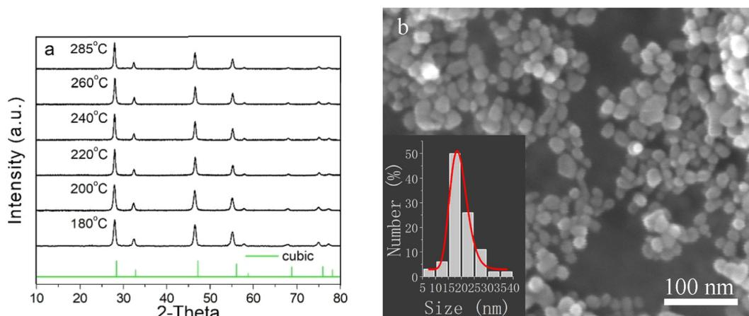
Fig. 1 XRD results of  $\text{NaYF}_4\text{:Yb, Er}$  NPs prepared at 180 °C, 200 °C, 220 °C, 240 °C, 260 °C, and 285 °C (a). The JCPDS file number for the standard cubic bulk structure is 77-2042. FE-SEM image of the  $\text{NaYF}_4\text{:Yb, Er}$  UCNPs prepared at 285 °C (b). The histogram of the size distribution is shown in the inset.
