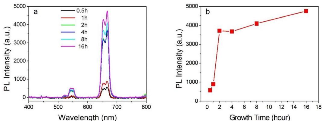
Fig. 3 Room-temperature UC luminescent spectra of NaYF<sub>4</sub>:20%Yb, 2%Er NPs prepared at different growth times (a). Relative PL intensity of the two-photon (<sup>4</sup>F<sub>9/2</sub>–<sup>4</sup>I<sub>15/2</sub>) 650 nm UC emission of Er ions vs. the growth time (b). Mass concentration of the NPs was kept constant at 2 mg mL<sup>-1</sup>. λ<sub>ex</sub> = 980 nm.
