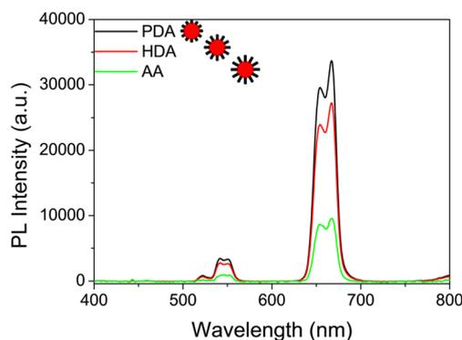
Fig. 4 Room-temperature UC luminescent spectra of  $\text{NaYF}_4:20\%\text{Yb}$ ,  $2\%\text{Er}$  NPs prepared with different chain length diacid ligands. Mass concentration of the NPs was kept constant at  $10 \text{ mg mL}^{-1}$ .  $\lambda_{\text{ex}} = 980 \text{ nm}$ .
