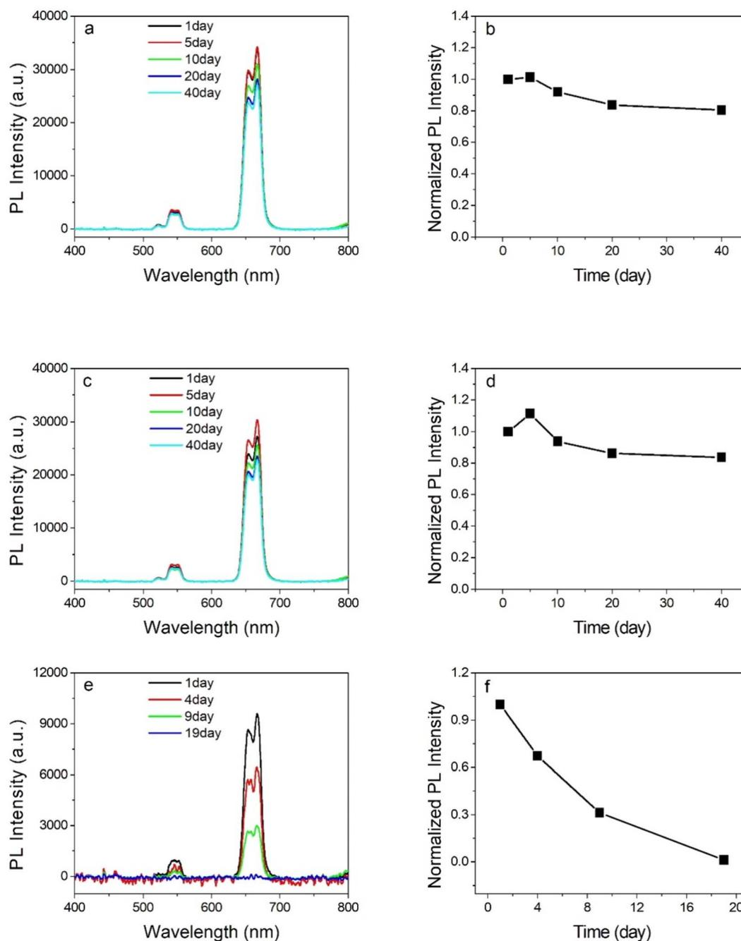
Fig. 5 Time evolution of room-temperature UC luminescent spectra and red emission intensity of NaYF<sub>4</sub>:20%Yb, 2%Er NPs prepared with PDA (a and b), HDA (c and d) and AA (e and f) under natural position to compare the stability of the relative NPs. Mass concentration of the NPs was kept constant at 10 mg mL<sup>-1</sup>.  $\lambda_{\text{ex}} = 980$  nm.
