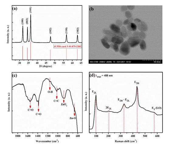
Fig. 1 Different room temperature characterizations of EZO sample. (a) XRD diffractogram. (b) TEM image. (c) FTIR transmitted light curve. (d) Raman spectrum recorded at 488 nm excitation wavelength.
