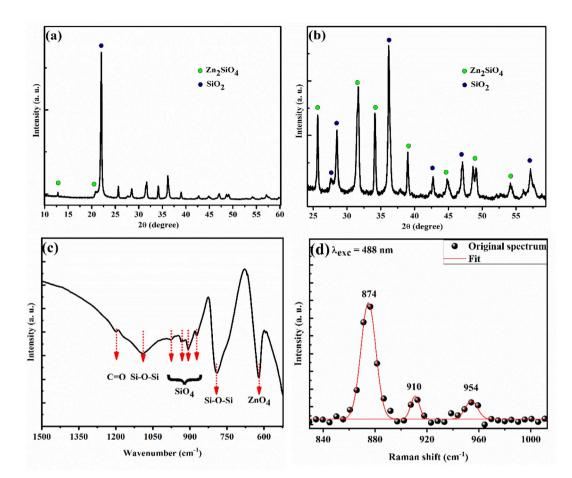
Fig. 2 Different characterizations of the EZS sample. (a) XRD diffractogram with different labels corresponding to silica and zinc silicate phases. (b) A close look into [23–60°] angular range of XRD graph. (c) FTIR transmitted light curve. (d) Raman spectrum recorded at 488 nm excitation wavelength.
