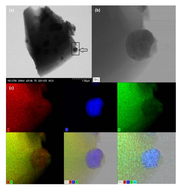
Fig. 3 Morphology of  $SiO_2/Zn_2SiO_4$ : Eu through TEM setup. (a)  $SiO_2/EZS$  composite. (b) Zoom of the mentioned frame. (c) Mapping element analysis of (b).
