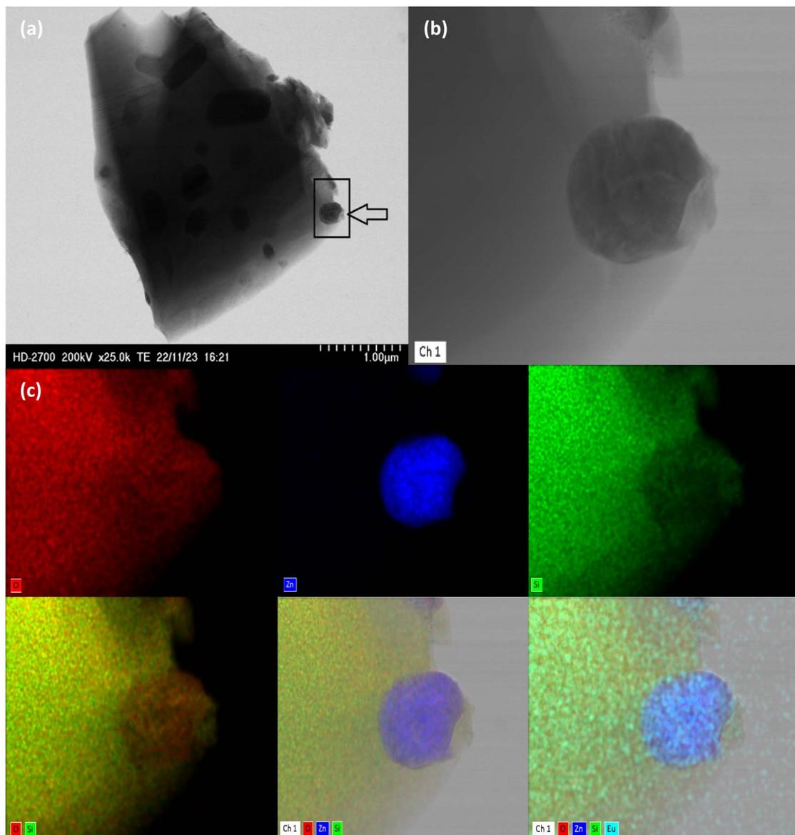
Fig. 3 Morphology of  $\text{SiO}_2/\text{Zn}_2\text{SiO}_4:\text{Eu}$  through TEM setup. (a)  $\text{SiO}_2/\text{EZS}$  composite. (b) Zoom of the mentioned frame. (c) Mapping element analysis of (b).
