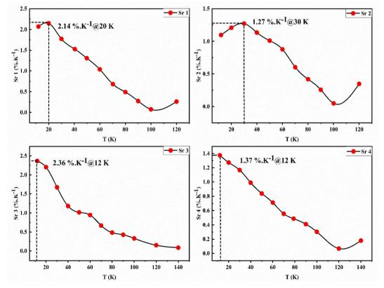
Fig. 6 Pattern of relative sensitivity ( $Sr_{1-4}$ ) versus temperature.
