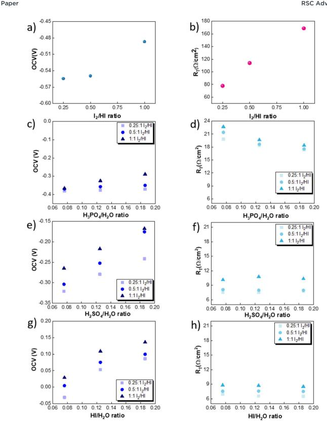
Fig. 4 Variation in the OCV for three  $I_2/HI$  ratios of 0.25, 0.5 and 1 for the catholytes (a)  $H_2O_4$ , (c)  $H_3PO_4$ , (e)  $H_2SO_4$ , and (g) HI. Variation in the  $R_T$ for the three  $I_2/HI$  ratios of 0.25, 0.5 and 1 for the catholytes (b)  $H_2O$  (d)  $H_3PO_4$  (f)  $H_2SO_4$  (h) HI.
