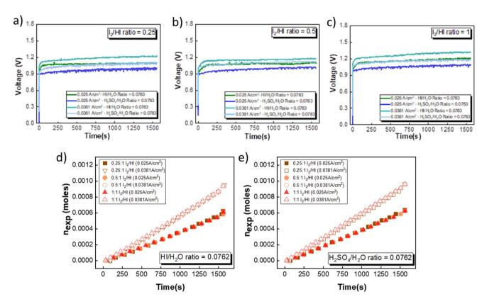
Fig. 7 Voltage evolution over time in an electrochemical HI decomposition experiment for three  $I_2$ /HI ratios is shown for (a) 1, (b) 0.5, and (c) 0.25 with HI and  $H_2SO_4$  as the catholyte. The hydrogen moles collected over time are shown for the two current densities for (d) HI and (e)  $H_2SO_4$ , respectively.
