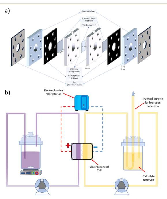
Fig. 1 Schematic representation of (a) the two-compartment electrochemical HI decomposition cell and (b) the continuous flow system for electrochemical HI decomposition.
