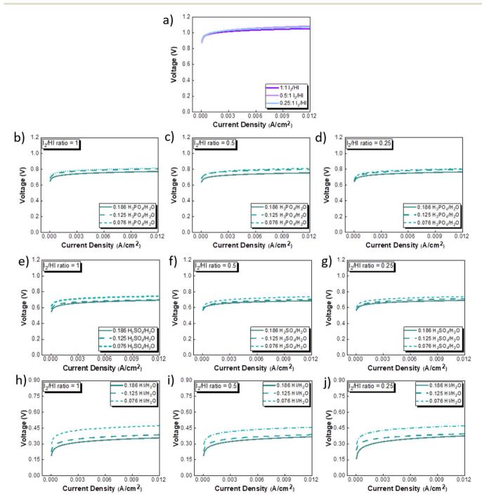
Fig. 5 Activation overpotential losses corresponding to the three  $I_2/HI$  ratios of 0.25, 0.5 and 1 with the catholytes (a)  $H_2O$  (b)-(d)  $H_3PO_4$  (e)-(g)  $H_2SO_4$ , and (h)-(j)  $H_1$ .
