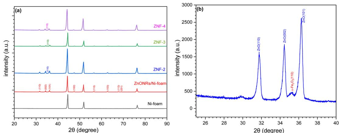
Fig. 4 (a) XRD patterns of Ni-foam, ZnO NRs/Ni-foam, (ZNF-2), (ZNF-3) and (ZNF-4). (b) High-resolution XRD pattern of ZNF-3.
