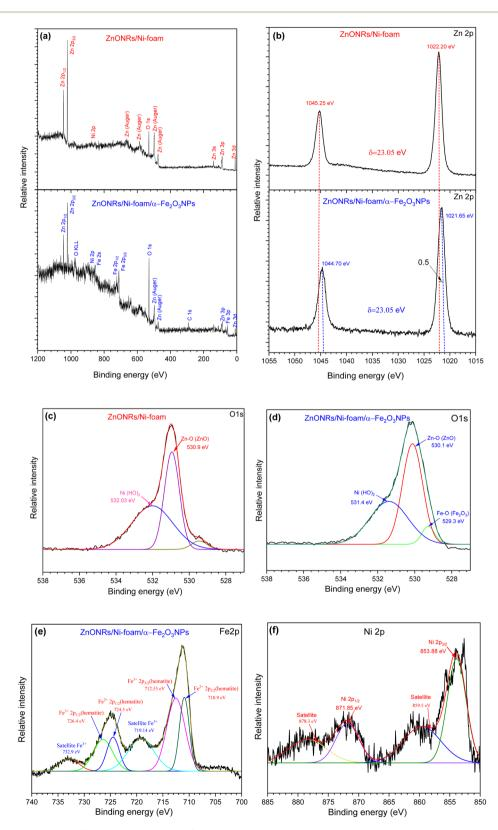
Fig. 5 XPS analysis of the ZnO NRs/Ni-foam and ZnO NRs/Ni-foam/ $\alpha$ -Fe<sub>2</sub>O<sub>3</sub> NPs nanocomposite: (a) survey spectra; high-resolution (b) Zn 2p, (c and d) O 1s, and (e) Fe 2p spectra; (f) Ni 2p spectrum of the nickel foam substrate.
