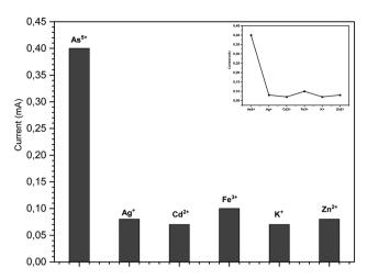
Fig. 7 Interference effect of different metal ions under similar experiment conditions used for the detection of arsenic(v) by the ZnO NRs/Ni-foam/ $\alpha$ -Fe<sub>2</sub>O<sub>3</sub>NP nanocomposite (50 ppb).
