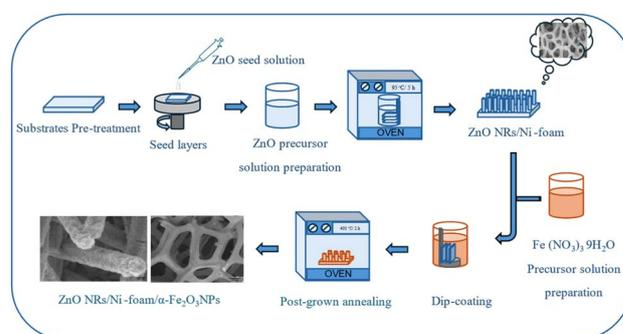
Fig. 1 Schematic showing the process for synthesis of the ZnO NRs/Ni-foam/ $\alpha$ -Fe<sub>2</sub>O<sub>3</sub>NPs nanocomposite electrode.
