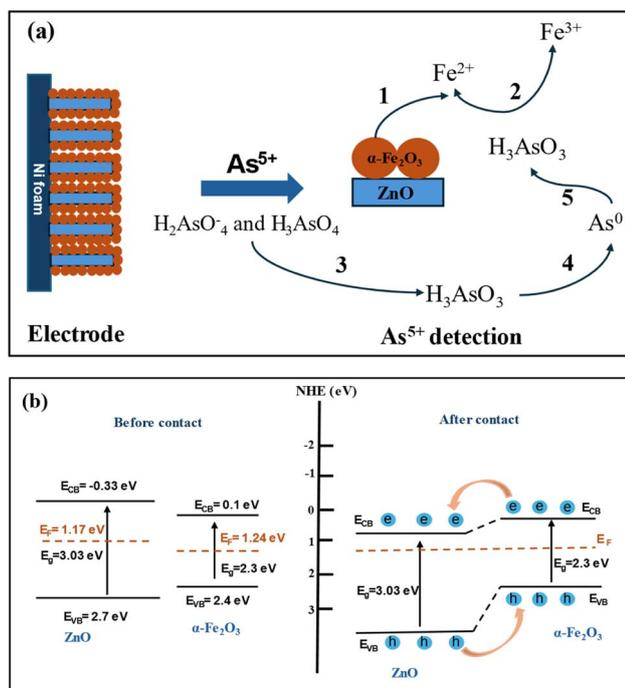
Fig. 8 (a) Schematic of the sensing mechanism (concept based on ref. 66) and (b) equilibrium energy band structure diagram of the ZnO NRs/Ni-foam/ $\alpha$ -Fe<sub>2</sub>O<sub>3</sub>NPs nanocomposite before and after contact between the ZnO NRs and  $\alpha$ -Fe<sub>2</sub>O<sub>3</sub>NPs.
