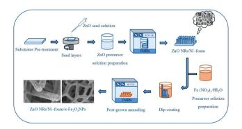
Fig. 1 Schematic showing the process for synthesis of the ZnO NRs/Ni-foam/ $\alpha$ -Fe<sub>2</sub>O<sub>3</sub>NPs nanocomposite electrode.
