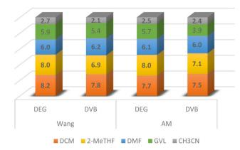
Fig. 3 Swelling (g mL<sup>-1</sup>) of DEG-PS vs. DVB-PS Wang and AM resins.
