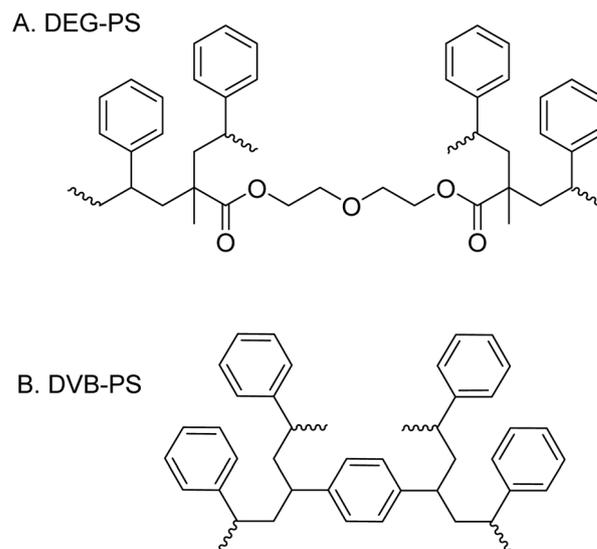
Fig. 1 Chemical structures of DEG-PS and DVB-PS resins.
