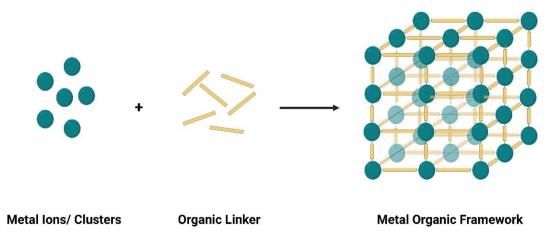
Fig. 6 Generic MOF composition from metal ions and organic linkers.
