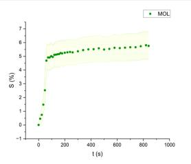
Fig. 8 Swelling curve of Methyl Oleate (MOL): percentage difference in surface area (S) over time with error band.
