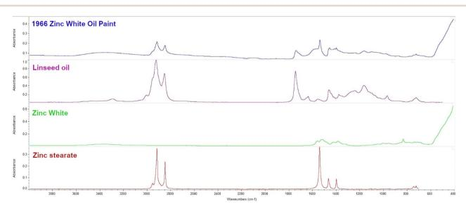
Fig. 2 FT-IR ATR spectra: comparison between the zinc white (ZnO) oil paint, linseed oil, zinc white, and zinc stearate.
