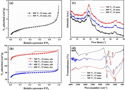
Fig. 2 Characterization of CCBC: BET (a and b); XRD patterns (c); and FTIR spectra (d).
