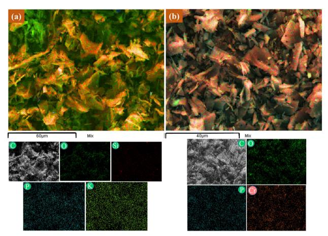
SEM-mapping of CCBC before (a) and after (b) Cr(vi) adsorption.
