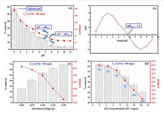
Fig. 3 The influence of pH on the adsorption of Cr(vI) onto CCBC (a); the isoelectric point of CCBC (b); adsorbent dosage (c) and ionic strength (d).
