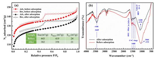
Fig. 5 N<sub>2</sub> adsorption–desorption at 77 K (a); FTIR spectra (b) of CCBC before and after Cr(vi) adsorption.
