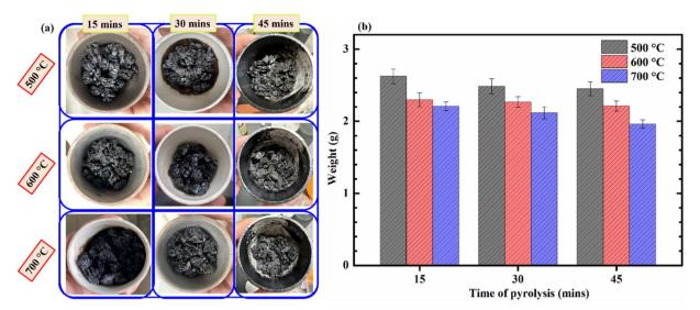
Fig. 1 Biochar products from corncobs (a); and the mass variation of biochar (b) under different pyrolysis conditions.
