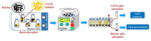
Scheme 2 Cr(vi) adsorption experiment onto corncob biochar.
