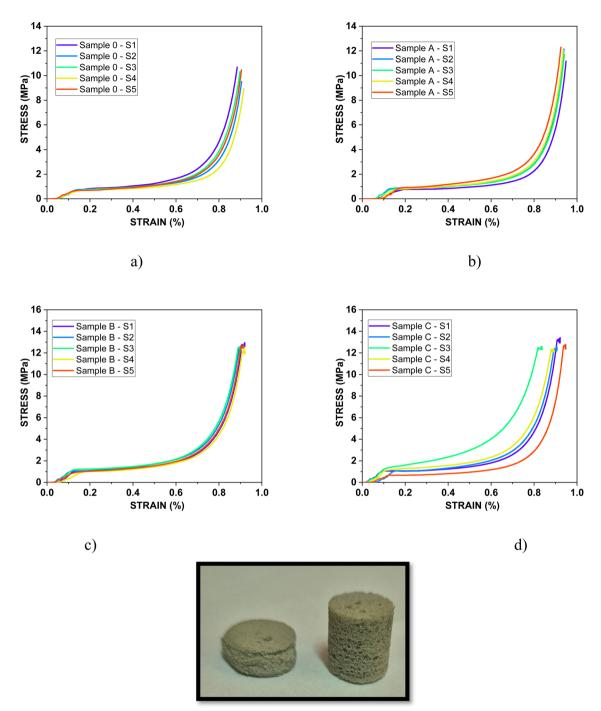
Fig. 7 Stress-strain plots for Samples 0, A, B, and C and the optical image of the sample recorded before and after the compression test.
