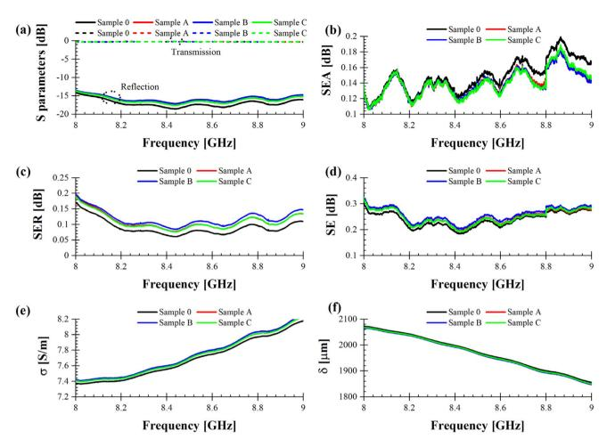
Fig. 11 (a) Measured S parameters. Extracted (b)  $SE_A$ , (c)  $SE_R$ , (d) SE, (e) conductivity, and (f) skin depth for blank PUR foam and the specimens loaded with MXenes in the 8-9 GHz band.
