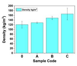
Fig. 5 Densities of the samples *versus* the MXenes content in the PUR foam specimens.
