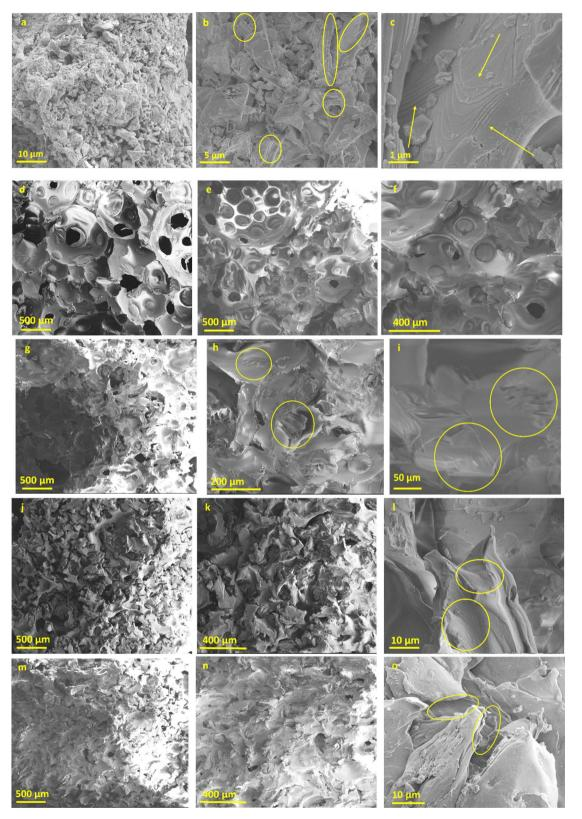
Fig. 2 SEM micrographs of Nb<sub>2</sub>AlC-MXenes (a, b, and c), blank sample (sample 0) in different areas (d, e, and f), Sample A loaded with 0.3 g MXenes (g, h, and i), Sample B loaded with 0.5 g MXenes (j, k, and l), respectively Sample C loaded with 0.7 g MXenes (m, n, and o); the yellow arrows indicate detailed micrographs of the folded MXenes (image c), while the yellow circles evidenced the presence of exfoliated MXenes embedded in the walls of the PUR foams (detail images i, l, and o).
