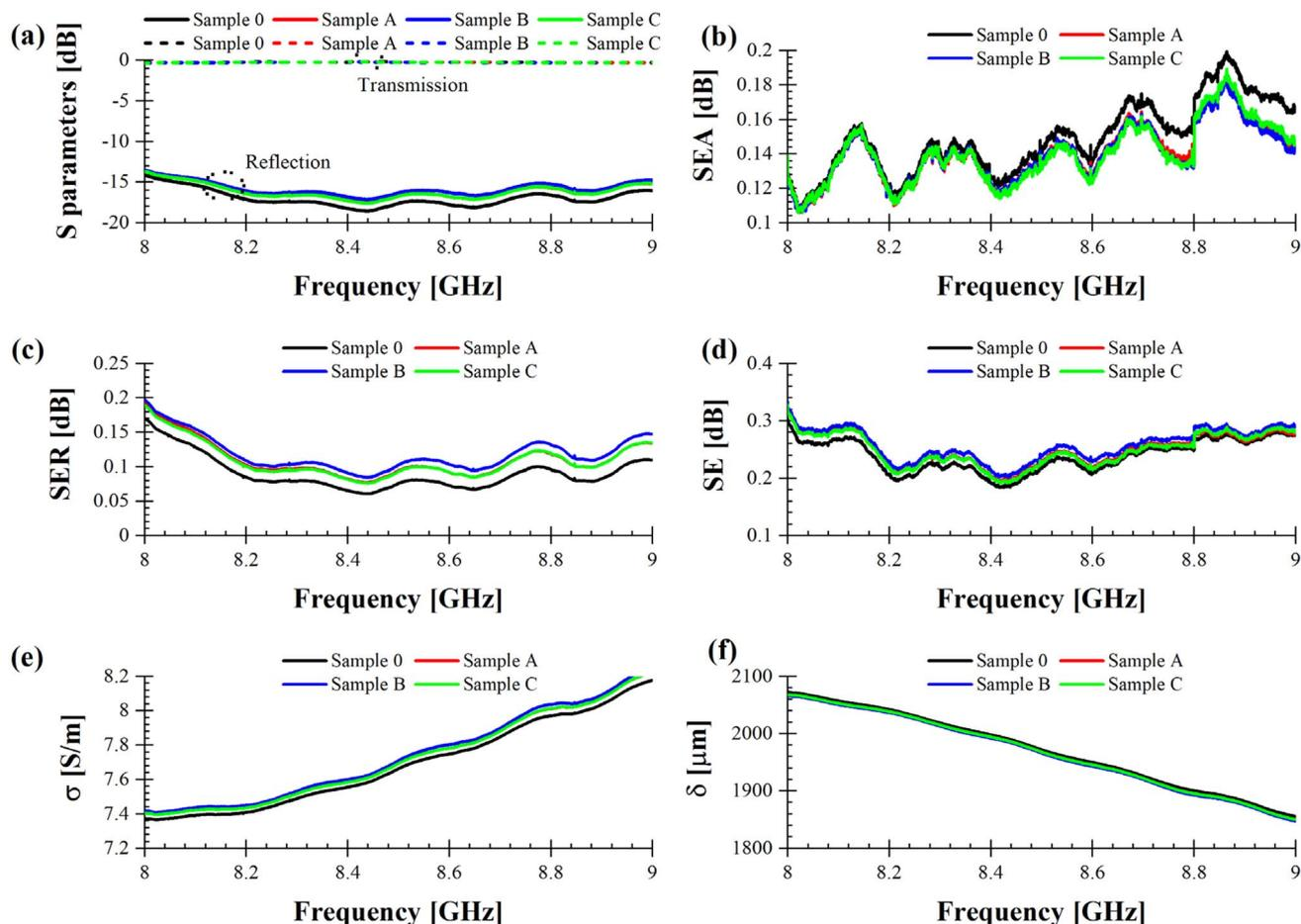
Fig. 11 (a) Measured  $S$  parameters. Extracted (b)  $SE_A$ , (c)  $SE_R$ , (d)  $SE$ , (e) conductivity, and (f) skin depth for blank PUR foam and the specimens loaded with MXenes in the 8–9 GHz band.
