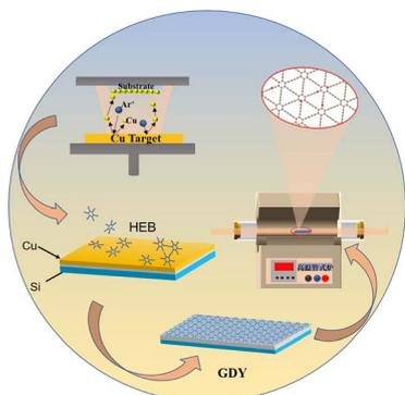
Fig. 1 Schematic diagram for the synthesis of N-GDY.
