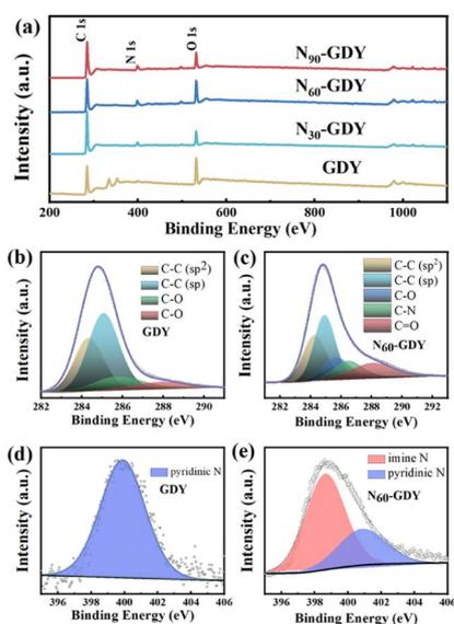
Fig. 4 (a) XPS spectra (survey) of  $N_{30}$ -GDY,  $N_{60}$ -GDY and  $N_{90}$ -GDY. (b) and (c) are XPS C 1s spectra of GDY and  $N_{60}$ -GDY, respectively. (d) and (e) is the XPS N 1s spectrum of GDY and  $N_{60}$ -GDY, respectively.
