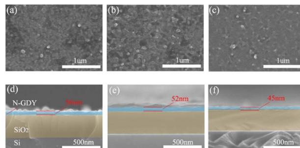
Fig. 2 (a–c) Exhibit the SEM morphologies of N<sub>30</sub>-GDY, N<sub>60</sub>-GDY, and N<sub>90</sub>-GDY samples, respectively. (d–f) Exhibit the cross-sectional SEM morphologies of N<sub>30</sub>-GDY, N<sub>60</sub>-GDY, and N<sub>90</sub>-GDY samples, respectively.
