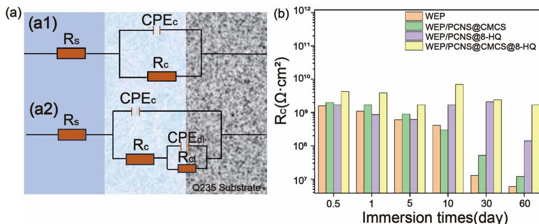
Fig. 7 (a) Equivalent electrical circuits (EEC) for EIS testing: (a1) Model 1, (a2) Model 2; (b)  $R_c$  values of WEP, WEP/PCNS@CMCS, WEP/PCNS@8-HQ, and WEP/PCNS@CMCS@8-HQ.
