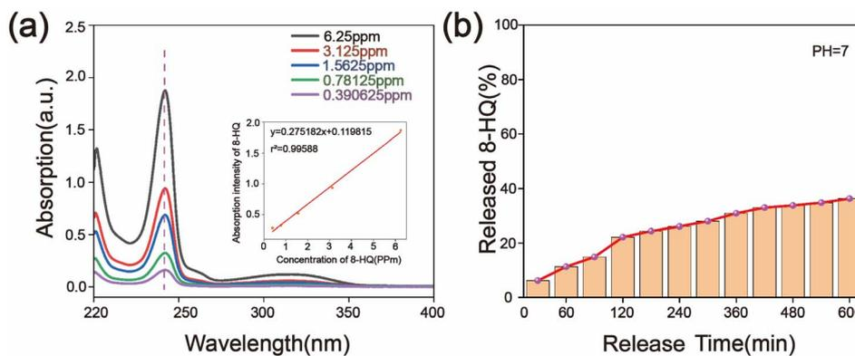
Fig. 5 (a) UV-vis spectra of 8-HQ solution and the corresponding standard curve; (b) release rate of 8-HQ from PCNS@CMCS@8-HQ in 3.5% NaCl solution.
