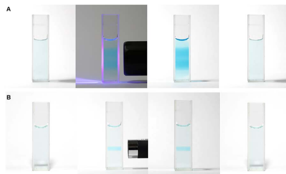
Fig. 2 Changes in the color of the solution: (A) blue-violet LED lamp; (B) blue-violet laser pointer. Photographic images (from left to right) show solutions before irradiation, during irradiation, 5 s after the end of irradiation, and 120 s after the end of irradiation.
