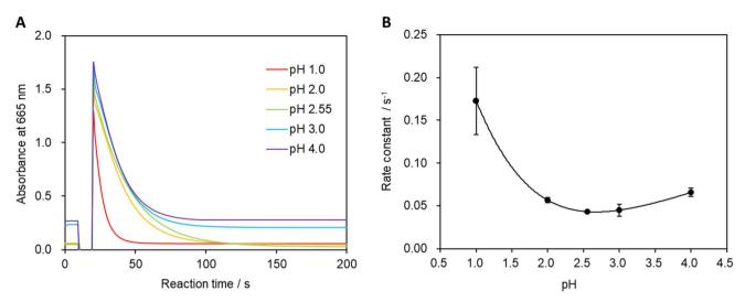
Fig. 6 (A) Absorbance at a wavelength of 665 nm. Absorbance measurements were performed 10 times, and the displayed values correspond to the solution that exhibited the median reaction rate constant. (B) Relationship between solution pH and reaction rate constant. Measurements were conducted 10 times, and error bars correspond to 99% confidence as determined using the Student's t-test.
