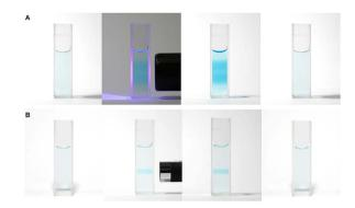
Fig. 2 Changes in the color of the solution: (A) blue-violet LED lamp; (B) blue-violet laser pointer. Photographic images (from left to right) show solutions before irradiation, during irradiation, 5 s after the end of irradiation, and 120 s after the end of irradiation.
