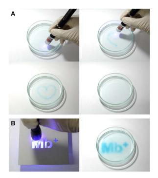
Fig. 10 Solution being painted and returning to a colorless state after approximately 90 s. (A) Blue-violet laser pointer; (B) blue-violet LED lamp.
