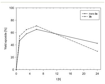
Fig. 7 Comparison of epoxide yields of complexes *trans-3a* and 3b (lines between measured points are just optical guidelines without physical meaning).
