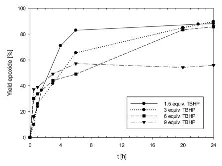
Fig. 5 Yield of epoxide with catalyst 1 with different amounts of TBHP (50 °C, CHCl<sub>3</sub>, 1 mol% 1; equiv. TBHP = molar equivalents to cyclooctene; lines between measured points are just optical guidelines without physical meaning).
