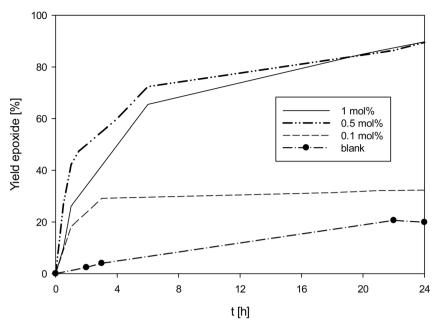
Fig. 6 Yield of epoxide with catalyst 1 at different catalyst loadings (50 °C, CHCl<sub>3</sub>, 3 equiv. TBHP; lines between measured points are just optical quidelines without physical meaning).
