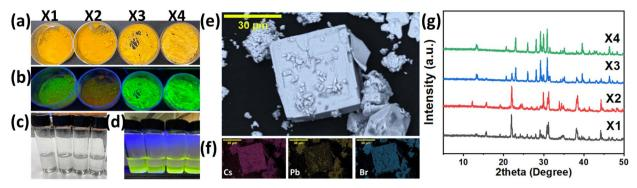
Fig. 1 Different caesium lead bromide perovskite powders prepared *via* grinding method: (a) under white light. (b) Under UV light. Their corresponding perovskites dissolved in DMSO (c) under white light. (d) Under U.V. light. (e) Scanning Electron Microscope (SEM) images of CsPbBr<sub>3</sub> perovskite. (f) Elemental mapping of perovskite elements: Cs, Pb, and Br. (g) Powder XRD patterns of caesium lead bromide perovskite powders.
