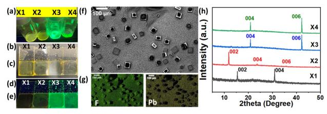
Fig. 2 (a) Perovskite/PVDF composites in (DMF/DMSO) mixed solvents under UV light. (b and d) Spin-coated thin films of perovskites only, and (c and e) perovskite/PVDF composites, under white and UV lights, respectively. (f) (SEM) images of  $CsPbBr_3/PVDF$  composite thin film and (g) its F and Pb elemental mapping. (h) XRD patterns of caesium lead bromide perovskites/PVDF composites thin films.
