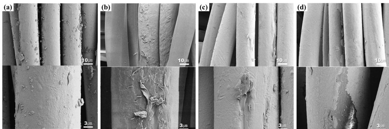
Fig. 9 SEM images of (a) before washed conductive fabric, (b) washed conductive fabric at 15 °C, (c) washed conductive fabric at 40 °C and (d) washed conductive at 60 °C ( $\times 3000$  &  $\times 10\,000$ ).
