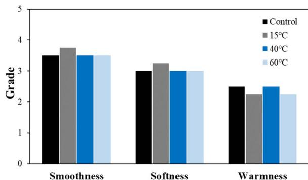
Fig. 12 Total hand value of the washed conductive fabrics according to washing temperature.
