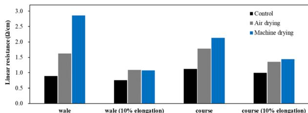
Fig. 16 Linear resistant according to drying method.
