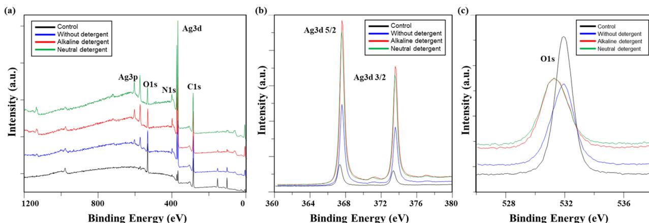
**Fig. 4** XPS of washed conductive fabrics according to detergent type: (a) a survey scan of XPS spectrum, high-resolution (b) Ag 3d, and (c) O 1s.
