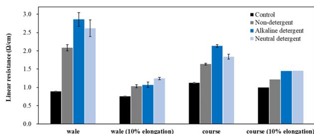
Fig. 6 Linear resistant according to detergent type.
