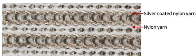
Fig. 1 Appearance of the conductive fabric (magnification: ×140).
