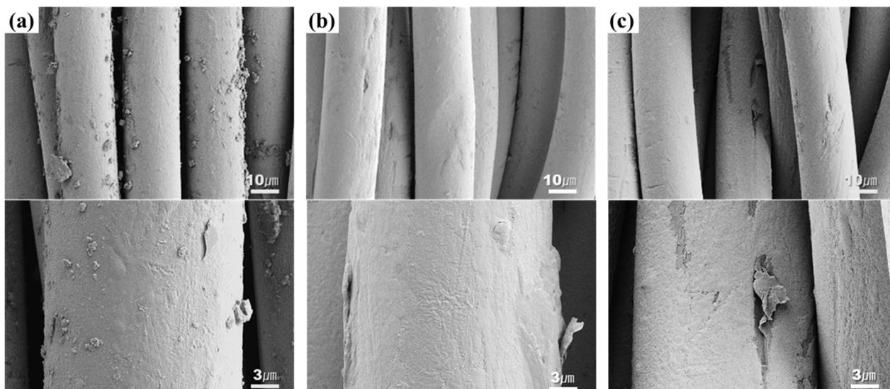
Fig. 14 SEM images of (a) before washed conductive fabric, (b) washed and air-dried conductive fabric, (c) washed and machine-dried conductive fabric ( $\times 3000$  &  $\times 10\,000$ ).
