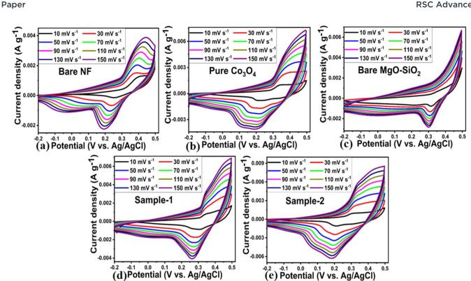
Fig. 6 CV polarization curves at different sweeping rates in 3 M KOH agueous solution of (a) bare nickel foam, (b) pure Co<sub>2</sub>O<sub>4</sub>, (c) bare MgO-SiO<sub>2</sub> (d) Co<sub>3</sub>O<sub>4</sub>/MgO-SiO<sub>2</sub> composite (sample 1), (e) Co<sub>3</sub>O<sub>4</sub>/MgO-SiO<sub>2</sub> composite (sample 2).
