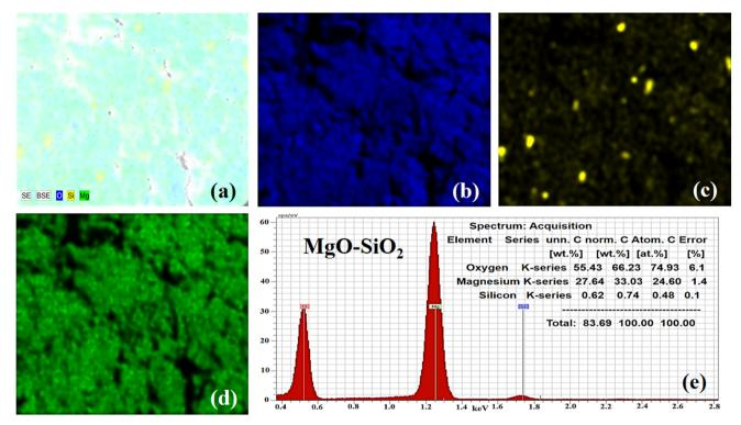
Fig. 3 (a) Elemental mapping of MgO-SiO<sub>2</sub>. (b-d) Elemental mapping of Mg, Si, and O. (e) EDX spectrum of the bare MgO-SiO<sub>2</sub> composite.
