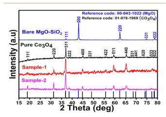
Fig. 1 XRD reflection peaks of pure  $Co_3O_4$ , bare  $MgO-SiO_2$  and  $Co_3O_4/MgO-SiO_2$  composites (sample 1 and sample 2).
