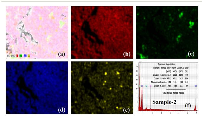
Fig. 4 (a) Elemental mapping of the  $Co_3O_4/MgO-SiO_2$  composite (sample 2). (b-e) Elemental mapping of O, Mg, Co, and Si of the  $Co_3O_4/MgO-SiO_2$  composite (sample 2). SiO<sub>2</sub> composite (sample 2). (f) EDX spectrum of the Co<sub>3</sub>O<sub>4</sub>/MgO-SiO<sub>2</sub> composite (sample 2).
