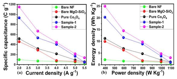
Fig. 8 (a) Specific capacitance calculations of the bare nickel foam, pure  $Co_3O_4$ , bare  $MgO-SiO_2$ ,  $Co_3O_4/MgO-SiO_2$  composite (sample 1), and  $Co_3O_4/MgO-SiO_2$  composite (sample 2) using GCD cycles at different current densities. (b) Energy and power density of specific capacitance calculations of pure  $Co_3O_4$ , bare  $MgO-SiO_2$ ,  $Co_3O_4/MgO-SiO_2$  composite (sample 1), and  $Co_3O_4/MgO-SiO_2$  composite (sample 2).
