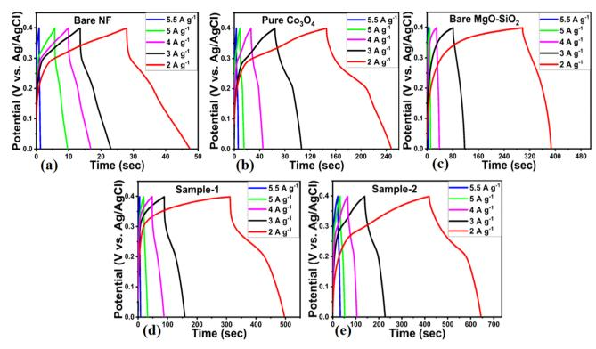
Fig. 7 GCD cycles measured at different current densities in 3 M KOH aqueous solution for (a) the bare nickel foam, (b) pure  $Co_3O_4$ , (c) bare  $MgO-SiO_2$  (d)  $Co_3O_4/MgO-SiO_2$  composite (sample 1), and (e)  $Co_3O_4/MgO-SiO_2$  composite (sample 2).
