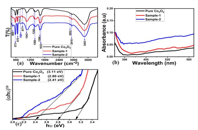
Fig. 5 Distinctive FTIR spectra of (a) pure  $Co_3O_4$  and  $Co_3O_4/MgO-SiO_2$  composites (sample 1 and sample 2), (b) UV-visible spectra of pure  $Co_3O_4$  and  $Co_3O_4/MgO-SiO_2$  composites (sample 1 and sample 2), and (c) corresponding Tauc plots of pure  $Co_3O_4$  and  $Co_3O_4/MgO-SiO_2$  composites (sample 1 and sample 2).
