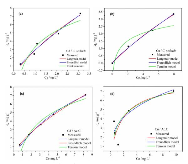
Fig. 6 Fitting of the adsorption isotherms for  $Cd^{2+}$  and  $Cu^{2+}$  ions using *Cystoseira sedoide* (a and b) and the industrial activated carbon (c and d).
