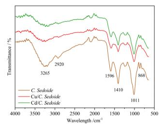
Fig. 2 FTIR spectra of *C. sedoide* powder before (brown curve) and after Cd<sup>2+</sup> (green curve) and Cu<sup>2+</sup> (red curve) biosorption.
