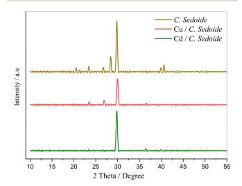
Fig. 1 XRD patterns of C. sedoide powder before (brown curve) and after  $Cd^{2+}$  (green curve) and  $Cu^{2+}$  (red curve) biosorption.
