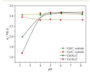
Fig. 4 Effect of solution pH on the adsorption capacity of  ${\rm Cd}^{2+}$  and  ${\rm Cu}^{2+}$  ions by *C. sedoide* and Ac.C.
