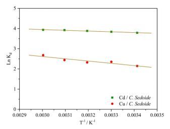
Fig. 9 Thermodynamic curves of  $Cd^{2+}$  and  $Cu^{2+}$  biosorption on Cystoseira sedoide alga.
