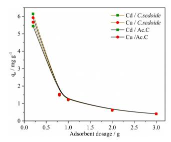
Fig. 3 Effect of C. sedoide alga and Ac.C doses on the adsorption capacity of  $Cd^{2+}$  and  $Cu^{2+}$  ions.
