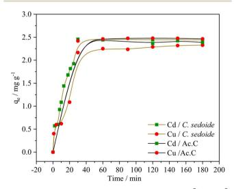
Fig. 7 Effect of contact time on adsorption capacity of Cd<sup>2+</sup> and Cu<sup>2+</sup> on Cystoseira sedoide and on activated carbon.
