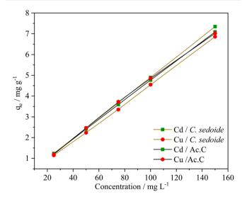
Fig. 5 Effect of  $Cd^{2+}$  and  $Cu^{2+}$  ions concentration on their adsorption capacity by *Cystoseira sedoide* and Ac.C.
