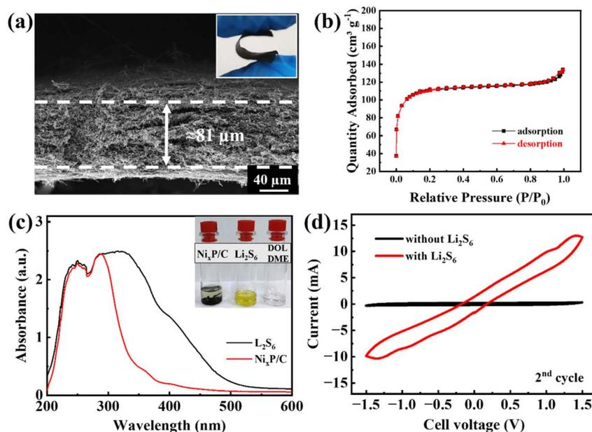
Fig. 3 Cross-sectional SEM (a), inset: digital image of flexibility,  $\text{N}_2$  adsorption-desorption isotherms (b) of the  $\text{Ni}_x\text{P}/\text{C}$  fiber mat (reproduced from ref. 25), UV-vis spectra after polysulfide adsorption test (c), inset: digital images of vials for polysulfide adsorption test, CV curves of symmetric cells with the  $\text{Ni}_x\text{P}/\text{C}$  fiber mats (d).
