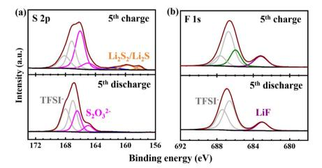
Fig. 6 S 2p (a) and F 1s (b) XPS spectra of the cathode side of the Ni<sub>x</sub>P/C interlayer after the 5th discharge and 5th charge at 0.2C in a lithium sulfur cell.
