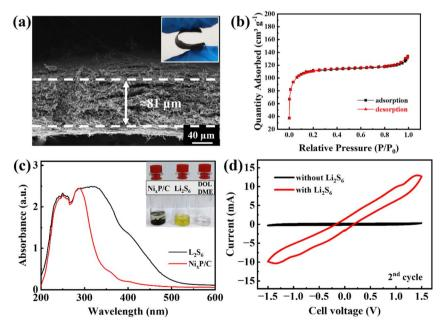
Fig. 3 Cross-sectional SEM (a), inset: digital image of flexibility,  $N_2$  adsorption—desorption isotherms (b) of the  $N_i$ P/C fiber mat (reproduced from ref. 25), UV-vis spectra after polysulfide adsorption test (c), inset: digital images of vials for polysulfide adsorption test, CV curves of symmetric cells with the  $N_i$ P/C fiber mats (d).
