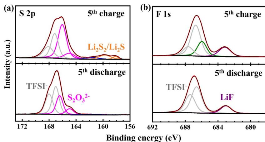
Fig. 6 S 2p (a) and F 1s (b) XPS spectra of the cathode side of the Ni<sub>x</sub>P/C interlayer after the 5th discharge and 5th charge at 0.2C in a lithium-sulfur cell.
