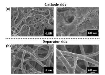
Fig. 7 FE-SEM images of the cathode side (a) and separator side (b) of the Ni<sub>x</sub>P/C interlayer after cycling at 0.2C.
