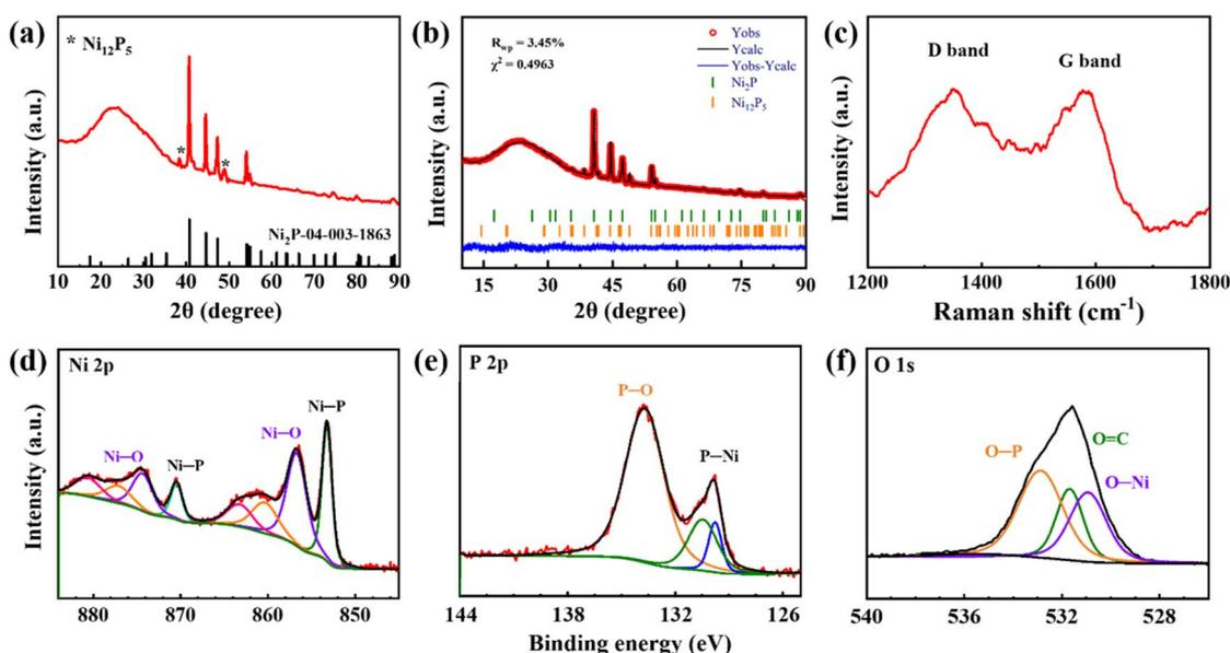
Fig. 1 XRD pattern (a), Rietveld refinement of XRD pattern (b), Raman spectrum (c), Ni 2p (d), P 2p (e), and O 1s (f) XPS spectra of prepared  $\text{Ni}_x\text{P}/\text{C}$  fiber mat. Adapted from ref. 25.
