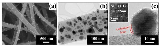
Fig. 2 Surface SEM (a), TEM (b), and HR-TEM (c) images of prepared Ni<sub>x</sub>P/C fiber mat. Inset: HR-TEM image with a lattice spacing. Adapted from ref. 25.
