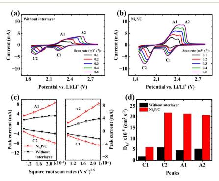
Fig. 4 Second CV curves of the GPC@S|Li cells at different scan rates without (a) and with (b) the Ni<sub>x</sub>P/C interlayer; peak currents (I<sub>n</sub>) vs. square root of scan rates ( $v^{0.5}$ ) (c) and comparison of calculated Li<sup>+</sup> diffusion coefficients (d).
