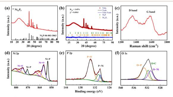
Fig. 1 XRD pattern (a), Rietveld refinement of XRD pattern (b), Raman spectrum (c), Ni 2p (d), P 2p (e), and O 1s (f) XPS spectra of prepared Ni<sub>x</sub>P/C fiber mat. Adapted from ref. 25.
