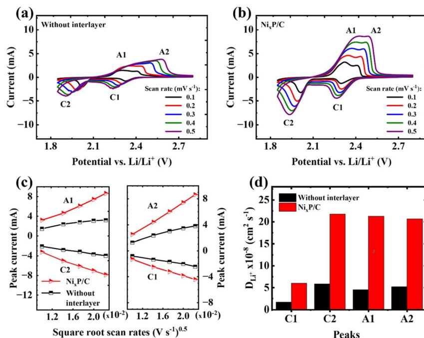
Fig. 4 Second CV curves of the GPC@S|Li cells at different scan rates without (a) and with (b) the Ni<sub>x</sub>P/C interlayer; peak currents ( $I_p$ ) vs. square root of scan rates ( $v^{0.5}$ ) (c) and comparison of calculated Li<sup>+</sup> diffusion coefficients (d).
