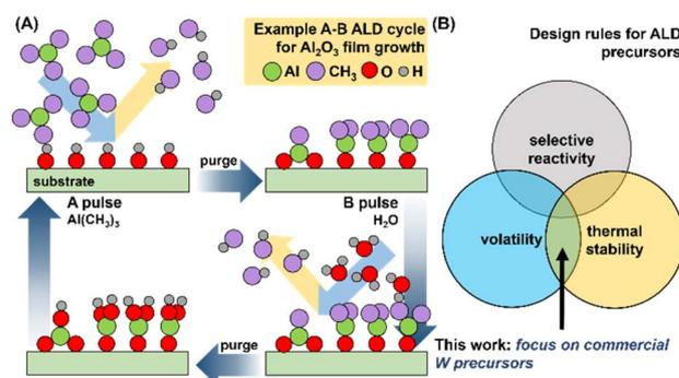
**Fig. 1** (A) Schematic representation of growth sequence for  $\text{Al}_2\text{O}_3$  film by ALD using  $\text{Al}(\text{CH}_3)_3$  and  $\text{H}_2\text{O}$  in an A–B cycle; an “ideal” ALD process. (B) Venn diagram of desirable characteristics for viable ALD precursors.
