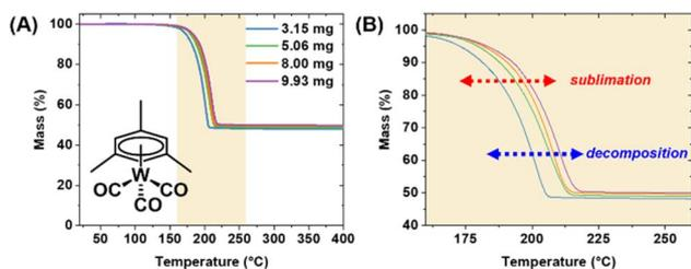
Fig. 5 (A) TGA traces of (mes)W(CO)<sub>3</sub> at varying masses with a temperature ramp rate of  $10\text{ }^\circ\text{C min}^{-1}$ . (B) Close up region where volatility is observed, highlighting overlapping sublimation and decomposition events.
