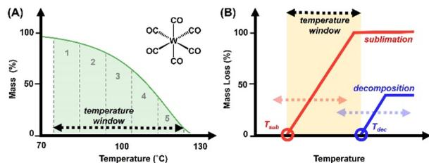
Fig. 2 (A) TGA trace of  $W(CO)_6$  with highlighted "TGA temperature window" and illustration of sequestered zones utilized for calculation of  $E_a$  and  $\Delta H_{sub}$ . (B) General schematic to illustrate the correlation of precursor volatility and stability juxtaposed against the potential ALD temperature window.
