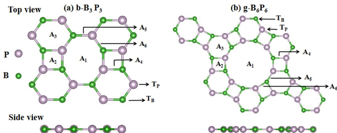
Fig. 1 Geometric structures of (a)  $\text{b-B}_3\text{P}_3$  and (b)  $\text{g-B}_6\text{P}_6$  sheets: top and side views with illustration of the available binding sites ( $A_1$ ,  $A_2$ ,  $A_3$ ,  $A_4$ ,  $A_5$ ,  $A_6$ ,  $T_B$  and  $T_P$ ).
