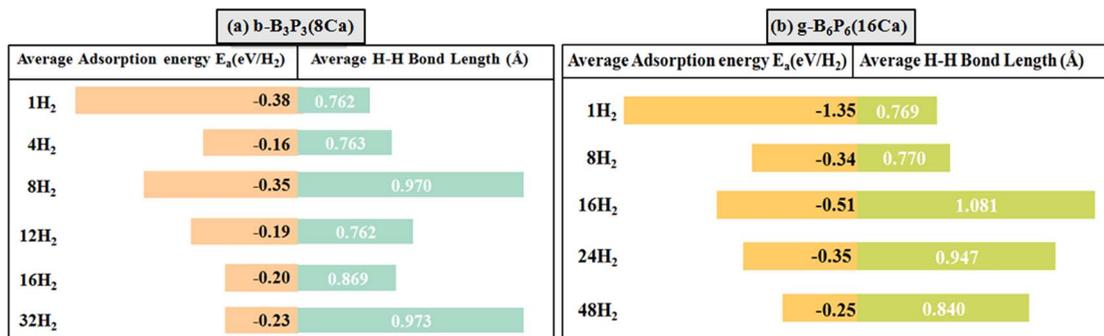
Fig. 4 The average  $E_a$  values (eV per H<sub>2</sub>) and average bond lengths (H–H) of H<sub>2</sub> molecules for (a) b-B<sub>3</sub>P<sub>3</sub>(8Ca) and (b) g-B<sub>6</sub>P<sub>6</sub>(16Ca). The lengths of the bars correspond to the  $E_a$  values.
