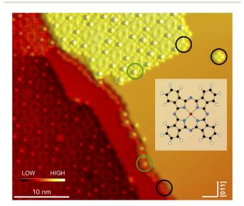
Fig. 1 Topograph of a submonolayer coverage of InPc on Pb(100) ( $V=200\,$  mV). The overview image covers three Pb terraces, which are separated by two monatomic steps. The molecules exhibit either a central depression or a protrusion. A few examples are indicated by black and green circles, respectively. The insert shows a schematic of InPc. White, black, blue, red dots represent hydrogen, carbon, nitrogen, and indium, respectively.
