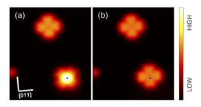
Fig. 7 Manipulation of an isolated molecule. Topographs (V = 500mV) showing two InPc molecules (a) before and (b) after applying V = $-3.1\,\mathrm{V}$  to the  $\uparrow$  molecule in the lower right corner. A small defect at the left edge of the image serves as a landmark. While the image of the upper molecule (1) remains unchanged the lower molecule is converted from ↑ to ↓.
