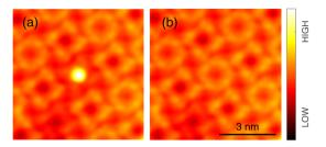
Fig. 8 Manipulation of a molecule in an island. Topographs (V = 200 mV) of an InPc island (a) prior to (b) after applying an elevated voltage V = -3.1 V to an InPc $\uparrow$  molecule at the centre of the image. After the manipulation, this molecule appears identical to the neighbouring InPc $\downarrow$  complexes.
