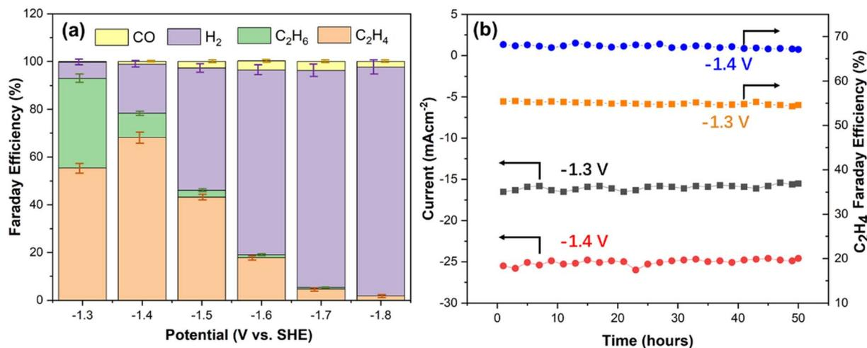
Fig. 5 (a) FE of the products generated by S10 at various potentials. (b) The FE of C<sub>2</sub>H<sub>4</sub> and current density of the CO<sub>2</sub> ERR using the S10 catalyst at -1.3 V and -1.4 V vs. SHE, respectively.
