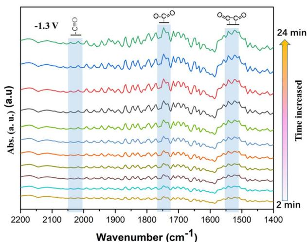
Fig. 6 Electrochemical *in situ* FTIR spectra of the S10 Cu-Cu<sub>2</sub>O/rGO at a potential of -1.3 V vs. SHE. All the spectra were subtracted from the initial one (recorded after activation of 100 s).
