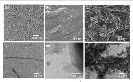
Fig. 1 (a) SEM image of CHNs/GO prepared from 125 mL CHNs and 1 mL 2 mg mL $^{-1}$  GO. (b and c) SEM images of the sample S10 Cu $^{-}$ Cu $^{2}$ O/rGO after *in situ* electrochemical reduction. (d) The TEM image of CHNs. (e) TEM image of CHNs/GO. (f) TEM image of Cu $^{-}$ Cu $^{2}$ O/rGO.
