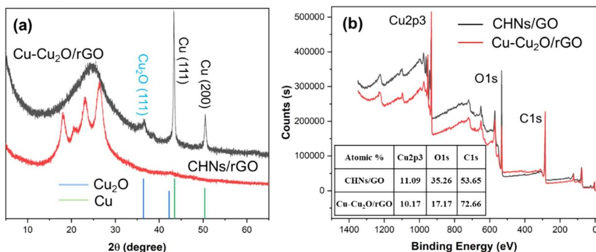
Fig. 3 (a) The XRD patterns and (b) survey scan XPS spectra of S10 before (CHNs/GO) and after electro-reduction (Cu–Cu<sub>2</sub>O/rGO). The inset table in (b) lists the atomic ratio of Cu, O, and C of S10 before and after electro-reduction, calculated from the XPS results.
