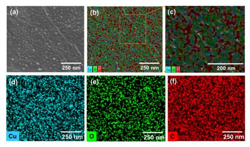
Fig. 2 (a) SEM image of S10 Cu-Cu<sub>2</sub>O/rGO with EDS mapping. The corresponding EDS mapping images; (b) overall elements combined together; (c) enlarged section of (b); (d) Cu, (e) oxygen and (f) carbon.
