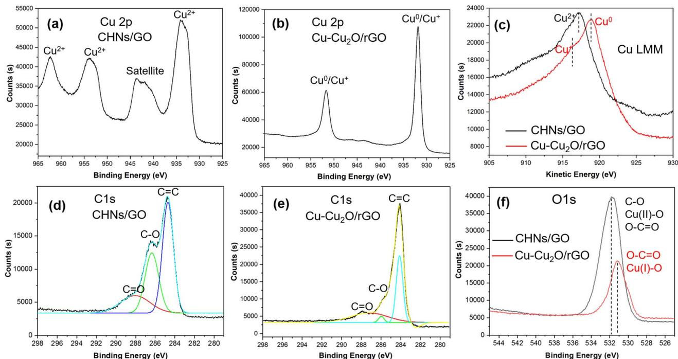
Fig. 4 High resolution XPS spectra of (a and b) Cu 2p, (c) Cu LMM, (d and e) C 1s; (f) O 1s of S10 before (CHNS/GO) and after (Cu-Cu<sub>2</sub>O/rGO) electro-reduction.
