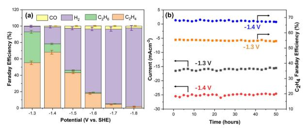
Fig. 5 (a) FE of the products generated by S10 at various potentials. (b) The FE of  $C_2H_4$  and current density of the  $CO_2$  ERR using the S10 catalyst at -1.3 V and -1.4 V vs. SHE, respectively.
