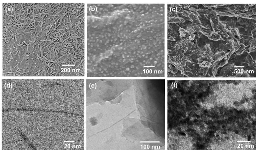
Fig. 1 (a) SEM image of CHNs/GO prepared from 125 mL CHNs and 1 mL 2 mg mL<sup>-1</sup> GO. (b and c) SEM images of the sample S10 Cu–Cu<sub>2</sub>O/rGO after *in situ* electrochemical reduction. (d) The TEM image of CHNs. (e) TEM image of CHNs/GO. (f) TEM image of Cu–Cu<sub>2</sub>O/rGO.
