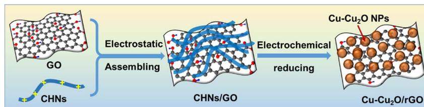
Scheme 1 Illustration of the synthesis process of Cu–Cu<sub>2</sub>O/rGO from CHNs/GO *via in situ* electrochemical deposition.
