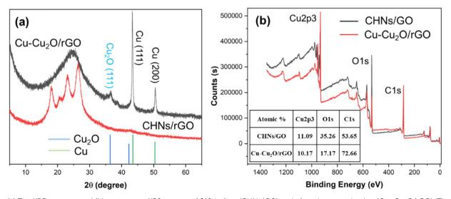
Fig. 3 (a) The XRD patterns and (b) survey scan XPS spectra of S10 before (CHNs/GO) and after electro-reduction (Cu-Cu<sub>2</sub>O/rGO). The inset table in (b) lists the atomic ratio of Cu, O, and C of S10 before and after electro-reduction, calculated from the XPS results.
