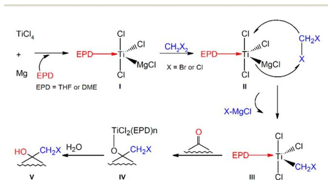
Fig. 1 The mechanism for  $\text{TiCl}_4$ -Mg mediated halomethylcarbinol formation proposed by Yan *et al.*<sup>32</sup>
