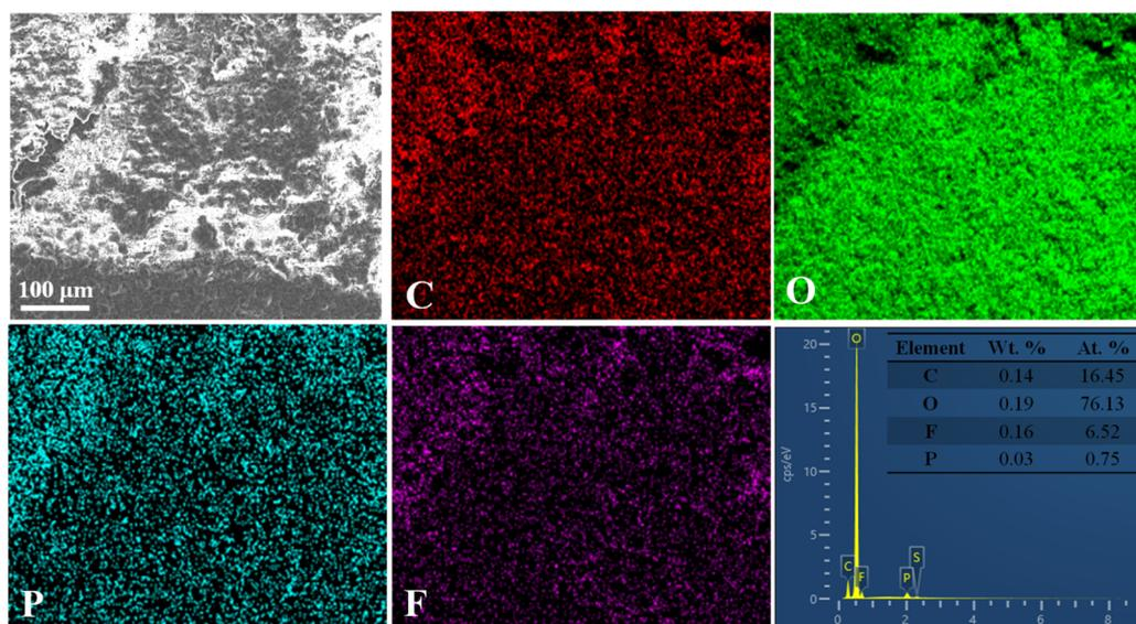
Fig. 4 The corresponding elemental mapping images for carbon, oxygen, phosphorus, fluorine and EDS spectrum of the Li foils obtained after 200 cycles in 1 M LiPF<sub>6</sub>/EC-EMC-DEC.
