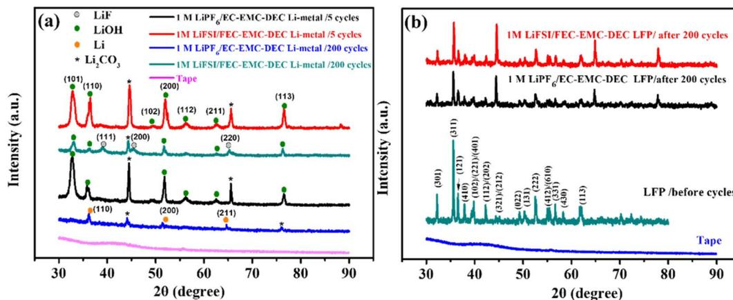
Fig. 7 XRD results of (a) Li-metal anodes after 5 and 200 cycles (b) and LiFePO<sub>4</sub> electrodes after 200 cycles in 1 M LiPF<sub>6</sub>/EC-EMC-DEC and 1 M LiFSI/FEC-EMC-DEC.
