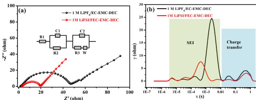
Fig. 6 (a) Nyquist plots and (b) DRT profiles of the Li||LiFePO<sub>4</sub> cells with 1 M LiPF<sub>6</sub>/EC–EMC–DEC and 1 M LiFSI/FEC–EMC–DEC as electrolytes.
