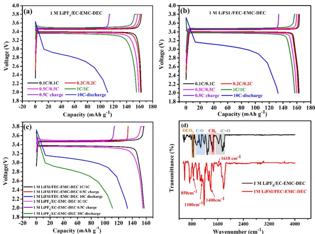
Fig. 2 Galvanostatic charge/discharge curves of Li||LiFePO<sub>4</sub> cells with (a) 1 M LiPF<sub>6</sub>/EC-EMC-DEC and (b) 1 M LiFSI/FEC-EMC-DEC electrolytes at different current densities. (c) Comparison of the overpotential and (d) FTIR results of the Li-metal anodes obtained after 200 cycles in 1 M LiPF<sub>6</sub>/EC-EMC-DEC and from 1 M LiFSI/FEC-EMC-DEC.
