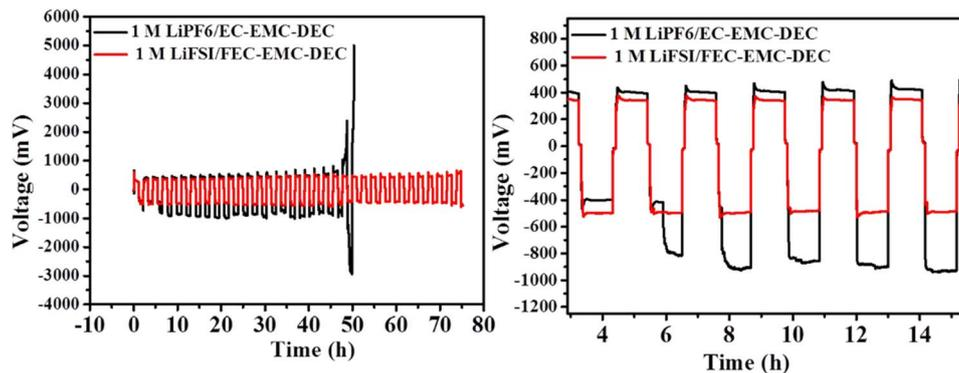
Fig. 9 The cycling performance of symmetrical cells with a Li metal anode in 1 M LiFSI/FEC-EMC-DEC and 1 M LiPF<sub>6</sub>/EC-EMC-DEC electrolytes at 0.5 mA cm<sup>-2</sup>.
