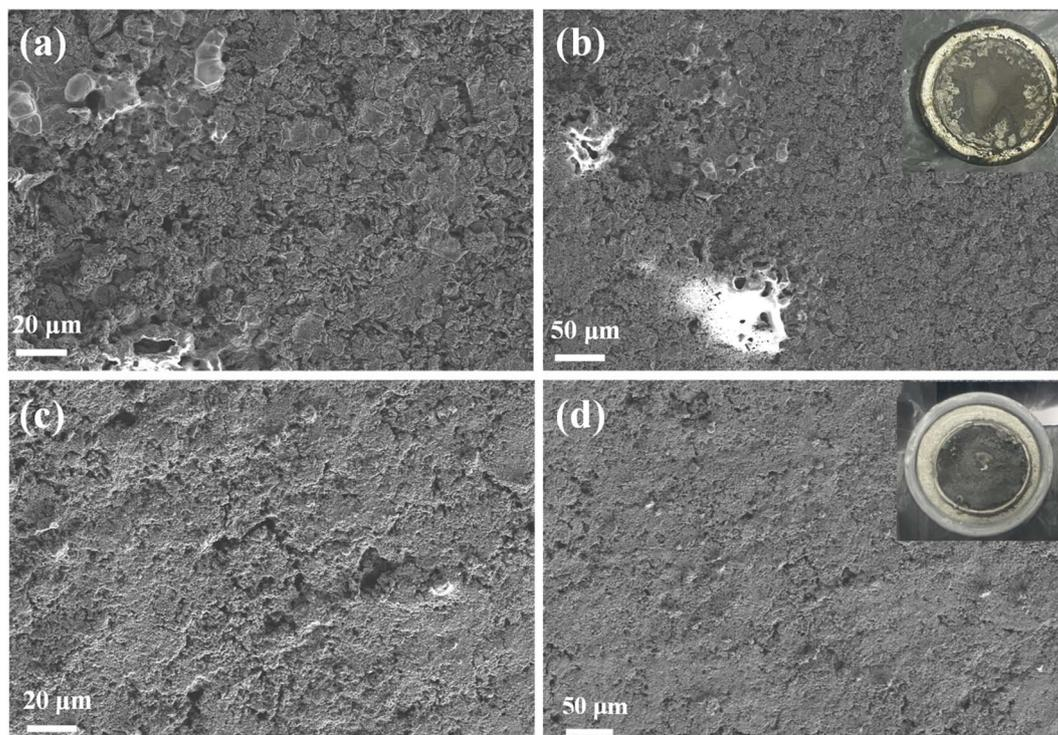
Fig. 3 SEM images of Li-metal anodes after 200 cycles in (a and b) 1 M LiPF<sub>6</sub>/EC-EMC-DEC and (c and d) 1 M LiFSI/FEC-EMC-DEC. The insets in (b) and (d) show the optical images of the respective Li foils after 200 cycles.
