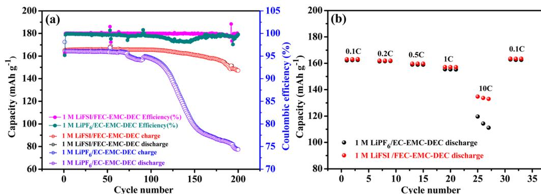
Fig. 1 (a) Cycle performance of Li||LiFePO<sub>4</sub> cells with 1 M LiFSI/FEC-EMC-DEC and 1 M LiPF<sub>6</sub>/EC-EMC-DEC as electrolytes at a current density of 1C (165 mA g<sup>-1</sup>). (b) Rate capability of Li||LiFePO<sub>4</sub> cells with 1 M LiFSI/FEC-EMC-DEC and 1 M LiPF<sub>6</sub>/EC-EMC-DEC as electrolytes at different current densities.
