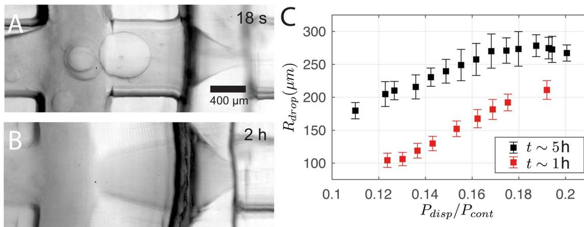
Fig. 10 (A and B) Deformation of the junction region of the chip that deforms under action of direct contact with the shell phase. (C) Single-emulsion droplet radius  $R_{\text{drop}}$  at different  $P_{\text{disp}}/P_{\text{cont}}$  generated at different times  $t$  of 1 hour and 5 hours of operation.
