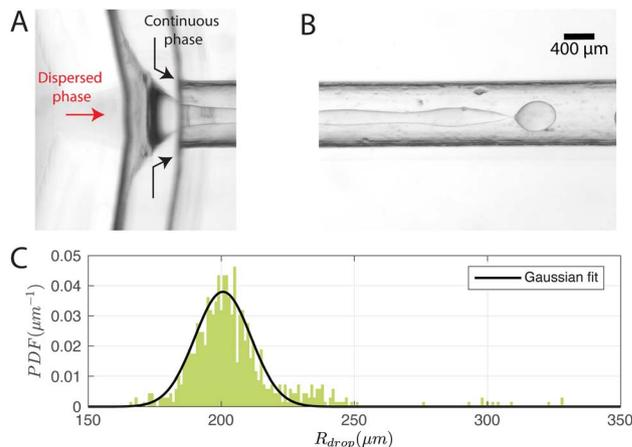
Fig. 4 Snapshot of (A) the junction and (B) the jet breaking up inside the chip when producing single-emulsion droplets with  $(P_{\text{disp}}, P_{\text{cont}}) = (9.5, 77.4)$  kPa. (C) Measured on-chip droplet size distribution and corresponding Gaussian fit.
