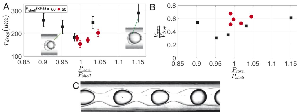
Fig. 8 Variation of (A) droplet size and (B) core-to-droplet volume fraction due to changes in core and shell phase pressures indicated in the legend. The marker colors correspond to different shell phase pressures. (C) Coaxial jet behavior above the maximum operating shell phase pressure, where core droplets are formed, but the coaxial jet does not break up inside the channel.  $P_{cont} = 75.4$  kPa is kept constant.
