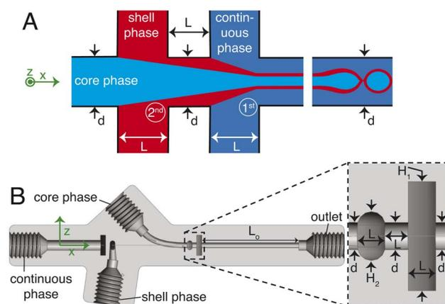
Fig. 1 (A) A sketch illustrating a double emulsion flow junction. (B) A SolidWorks® cross-section view of the droplet generator along the centreline.  $H_1 = 4$  mm,  $H_2 = 2$  mm,  $d = L = 1$  mm,  $L_o = 19$  mm. The coordinate system is shown in green.
