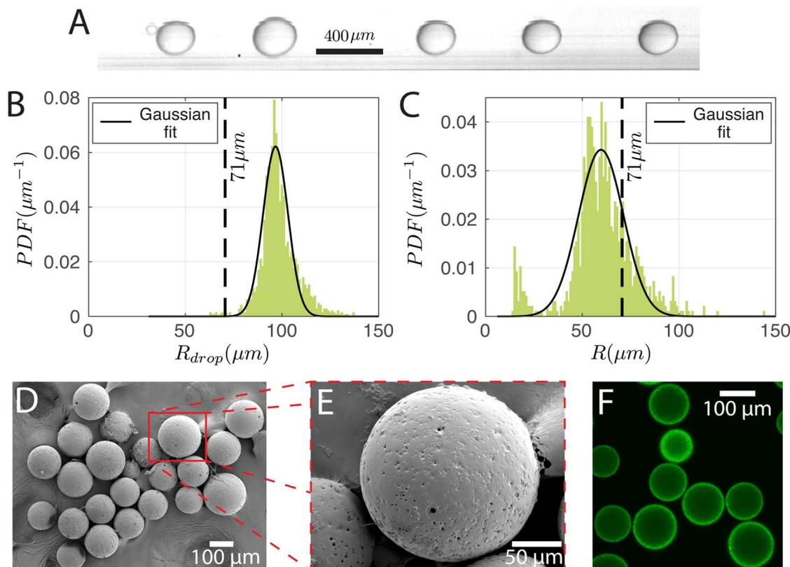
Fig. 6 (A) Image of the droplets in the chip before curing. Size distribution of (B) the droplets in the chip and (C) the cured particles with their Gaussian fits. (D) SEM image of the particles and (E) a zoomed image of a single particle. (F) Fluorescent image taken with confocal microscopy (excitation wavelength: 561 nm; detection wavelengths: 570 nm to 620 nm). The dashed lines in (B) and (C) indicate the calculated particle size assuming complete solvent evaporation.
