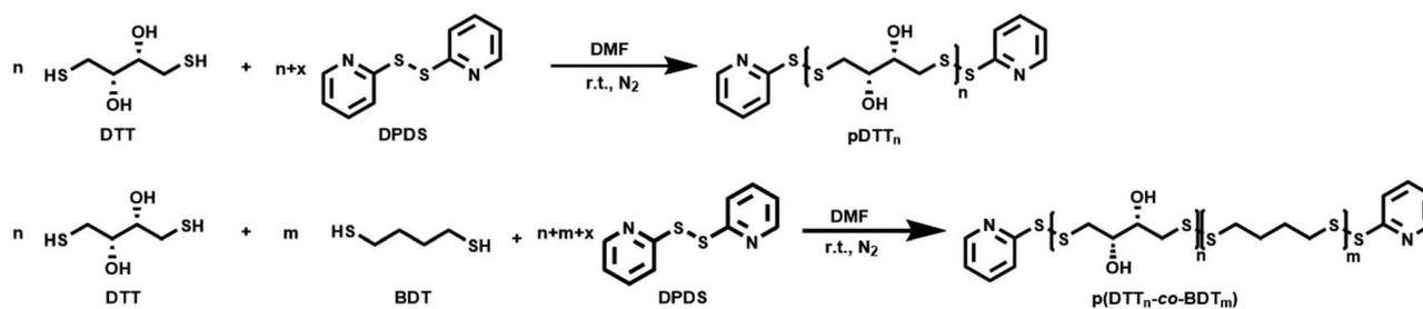
Scheme 1 Reaction scheme of the synthesis of homopolymer pDTT and copolymer p(DTT<sub>n</sub>-co-BDT<sub>m</sub>).
