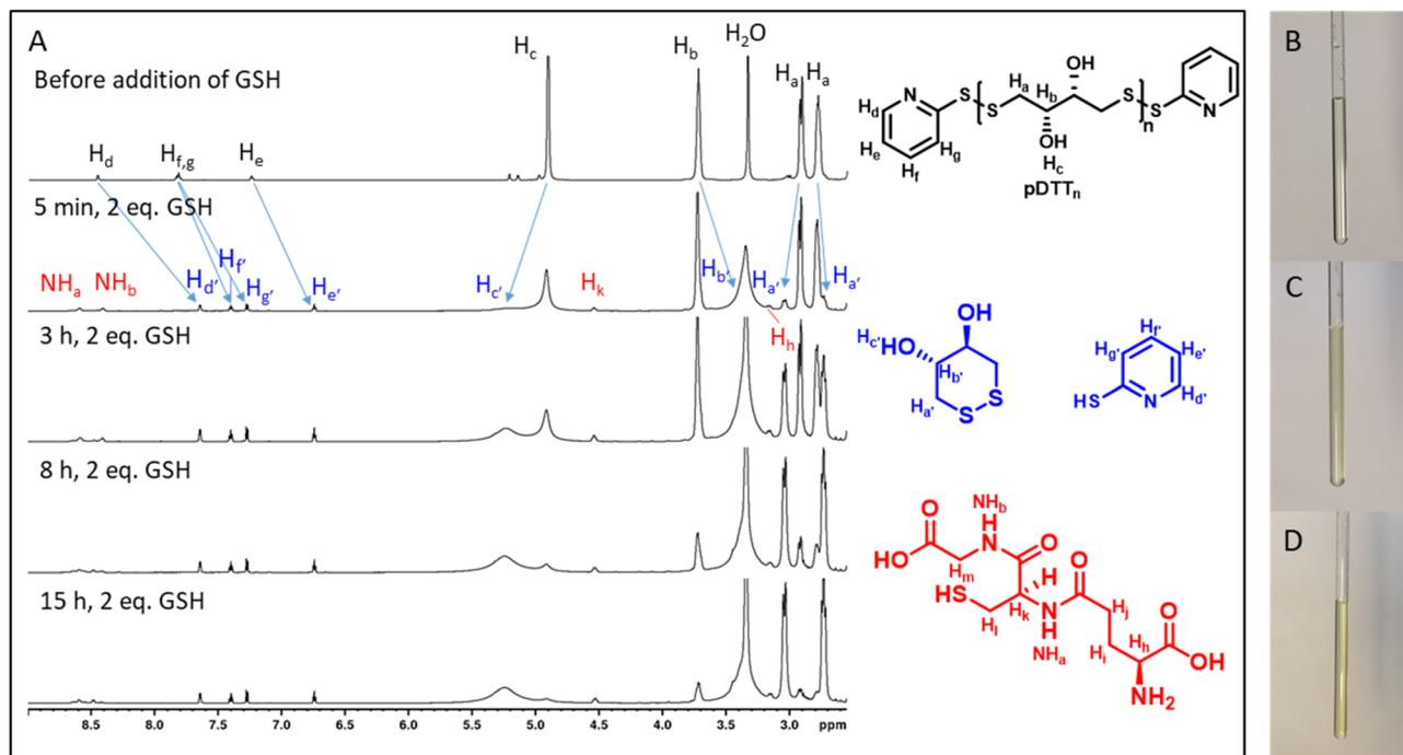
Fig. 2 Degradation of pDDT<sub>36</sub> with 2 eq. GSH (10.7 mM), <sup>1</sup>H-NMR spectra before and after addition of GSH (5 min, 3 h, 8 h, 16 h) (A), clear solution of pDDT<sub>36</sub> dissolved in d<sub>6</sub>-DMSO (B), turbid and light yellow solution of pDDT<sub>36</sub> dissolved in d<sub>6</sub>-DMSO immediately after addition of GSH (C), clear and yellow solution of pDDT<sub>36</sub> dissolved in d<sub>6</sub>-DMSO (D).
