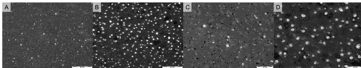
Fig. 5 pDTT<sub>36</sub> nanoparticles visualized by scanning electron microscopy at 5,000 $\times$  magnification without treatment, scale bar = 5  $\mu$ m (A) and after 24 h incubation with 10 mM glutathione, scale bar = 5  $\mu$ m (B). pDTT<sub>36</sub>-nanoparticles visualized by scanning electron microscopy at 10 000 $\times$  magnification without treatment scale bar = 2  $\mu$ m (C) and after 24 h incubation with 10 mM glutathione, scale bar = 2  $\mu$ m (D).
