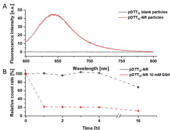
Fig. 7 Fluorescence of unloaded (blank) pD TT<sub>36</sub> particles and Nile red loaded particles (A); DLS count rate of pD TT<sub>36</sub> particles during incubation with or without GSH in relation to the initial value (B).
