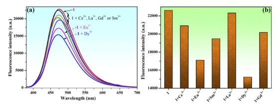
Fig. 10 Change in the fluorescence spectrum (a) and fluorescence intensity (b) of compound 1 ( $10^{-4}$  M) upon mixing with different rare earth metal ions (2 equivalents of La<sup>3+</sup>, Ce<sup>3+</sup>, Eu<sup>3+</sup>, Dy<sup>3+</sup>, Sm<sup>3+</sup> and Gd<sup>3+</sup>) in methanol–water (85:15, v/v) when  $\lambda_{ex} = 365$  nm.
