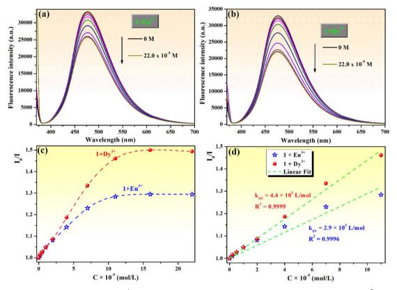
Fig. 11 Fluorescence spectra of compound 1 ( $10^{-4}$  M) upon addition of different concentrations (0-2.2 equivalents) of (a) Eu<sup>3+</sup> and (b) Dy<sup>3+</sup> ions. Stern–Volmer plots (c) and linear fit of Stern–Volmer plots in the concentration range of  $0-11 \times 10^{-5}$  M (d) for the interactions between compound 1 and Eu<sup>3+</sup> or Dy<sup>3+</sup> ions (at  $\lambda_{ex} = 365$  nm).
