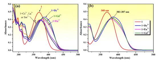
Fig. 9 (a) Change in the absorption spectrum of compound 1 ( $10^{-4}$  M) in the presence of different rare earth metal ions (5 equivalents of La<sup>3+</sup>  $Ce^{3+}$ ,  $Eu^{3+}$ ,  $Dy^{3+}$ ,  $Sm^{3+}$  and  $Gd^{3+}$ ) in methanol—water (85 : 15, v/v). (b) Details of absorption maximum shifts for phenolic Mannich base 1 (10<sup>-4</sup> M) upon addition of  $Eu^{3+}$ ,  $Dy^{3+}$  and  $Gd^{3+}$  ions (5 equivalents).
