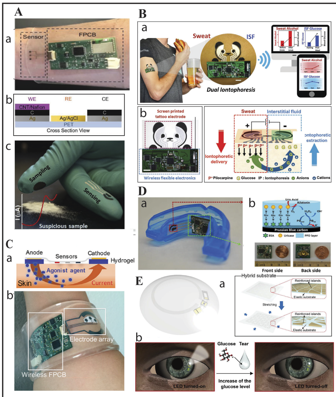
Fig. 1 Body wearable devices: (A) voltammetric sensors: (a) as sweat patch regulating the drug methylxanthine; (b) schematic of caffeine sensing band; and (c) fentanyl detecting gloves with square-wave voltammetry. Reproduced from ref. 6 with permission from Wiley-VCH, copyright 2018 & reproduced from ref. 7 with permission from Elsevier, copyright 2019. (B) Another wearable dual iontophoretic biosensor based on a tattoo, to simultaneously detect glucose and sweat: (a) dual iontophoretic biosensor for ISF glucose and sweat alcohol detection on a human subject with data being transmitted wirelessly to a mobile device; (b) screen printed electrode with wireless circuit on which the iontophoretic operation takes place. Reproduced from ref. 8 with permission from Wiley-VCH, copyright 2018. (C) Illustration of drug delivery via the iontophoretic technique: (a) and (b) showcase an integrated wristband for the detection of sweat via iontophoretic technique (sensors based on detecting cystic fibrosis electrochemically). Reproduced from ref. 9 with permission from the National Academy of Sciences, copyright 2017. (D) (a) Biosensor as a mouthguard with wireless circuit board integrated to an amperometric genosensor for detection of UA; (b) carbon WE modified with Prussian Blue attached to Uricase via BSA for detection of UA in saliva and photos showing wireless circuits from front and back side. Reproduced from ref. 10 with permission from Elsevier, copyright 2015. (E) (a) Schematics of a smart contact lens composed of a hybrid substrate which is embedded with stretchable conductors and functional devices to detect glucose in human tears in real-time; (b) schematics showing working of the lens by wireless transmission of power which activates the LED pixel and thus the sensor for detecting glucose. As the glucose level in the tear reaches a threshold level the LED pixel switches off. Reproduced from ref. 11 with permission from the American Association for the Advancement of Science, copyright 2018.
