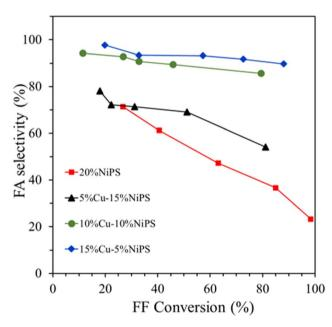
Fig. 7 Catalytic performance of the monometallic 20% NiPS and bimetallic Cu-NiPS catalysts toward the liquid-phase selective hydrogenation of FF to FA.
