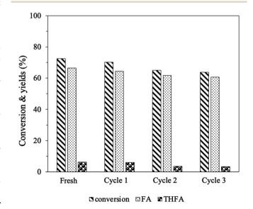
Fig. 8 Reusability test of the 15% Cu-5% NiPS catalyst used for the hydrogenation of FF to FA.
