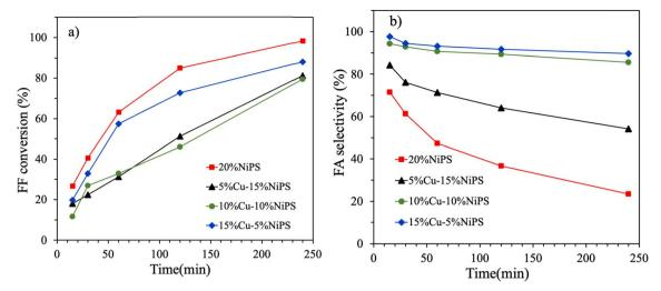
Fig. 6 The catalytic conversion of FF (a) and the selectivity to FA (b) in the liquid-phase selective hydrogenation of FF to FA on the monometallic 20% NiPS and bimetallic Cu-NiPS catalysts.
