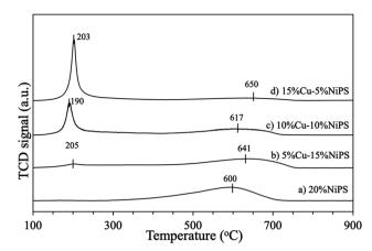
Fig. 4 H<sub>2</sub>-TPR profiles of catalysts (a) 20% NiPS, (b) 5% Cu-15% NiPS, (c) 10% Cu-10% NiPS, and (d) 15% Cu-5% NiPS.
