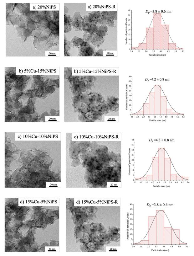
Fig. 3 TEM images and metal particle size distributions of the calcined and reduced catalysts: (a) 20% NiPS, (b) 5% Cu-15% NiPS, (c) 10% Cu-10% NiPS, and (d) 15% Cu-5% NiPS.
