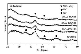
Fig. 1 XRD patterns of monometallic 20% NiPS and bimetallic Cu-NiPS catalysts (a) calcined at 400  $^{\circ}\text{C}$  and (b) reduced at 600  $^{\circ}\text{C}$ .
