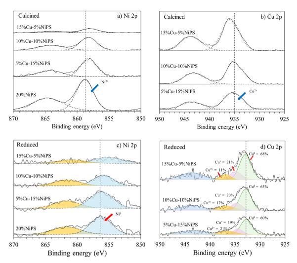
Fig. 5 XPS spectra: (a) Ni 2p and (b) Cu 2p of the calcined catalysts; (c) Ni 2p and (d) Cu 2p of the reduced catalysts.
