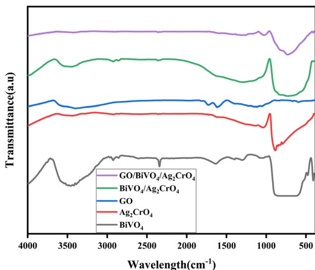
Fig. 5 Fourier transform infrared (FTIR) spectra of the fabricated  $\text{BiVO}_4$ ,  $\text{Ag}_2\text{CrO}_4$ ,  $\text{BiVO}_4/\text{Ag}_2\text{CrO}_4$ , GO and  $\text{GO}/\text{BiVO}_4/\text{Ag}_2\text{CrO}_4$  nanocomposites.
