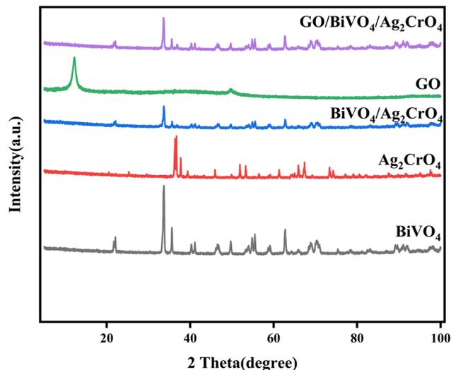
Fig. 1 XRD of the fabricated  $\text{BiVO}_4$ ,  $\text{Ag}_2\text{CrO}_4$ ,  $\text{BiVO}_4/\text{Ag}_2\text{CrO}_4$  and  $\text{GO}/\text{BiVO}_4/\text{Ag}_2\text{CrO}_4$  heterojunction photocatalysts.
