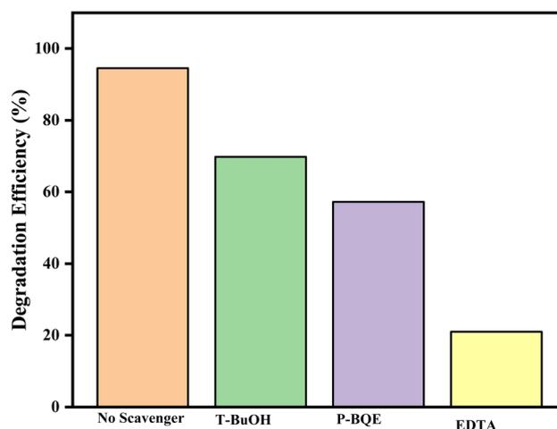
Fig. 13 Detection of reactive species with GO/BiVO<sub>4</sub>/Ag<sub>2</sub>CrO<sub>4</sub> composites during the ciprofloxacin degradation process.
