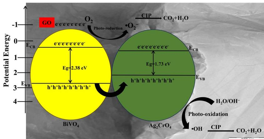
Fig. 15 Possible mechanism for ciprofloxacin photodegradation by the GO/BiVO<sub>4</sub>/Ag<sub>2</sub>CrO<sub>4</sub> photocatalyst.
