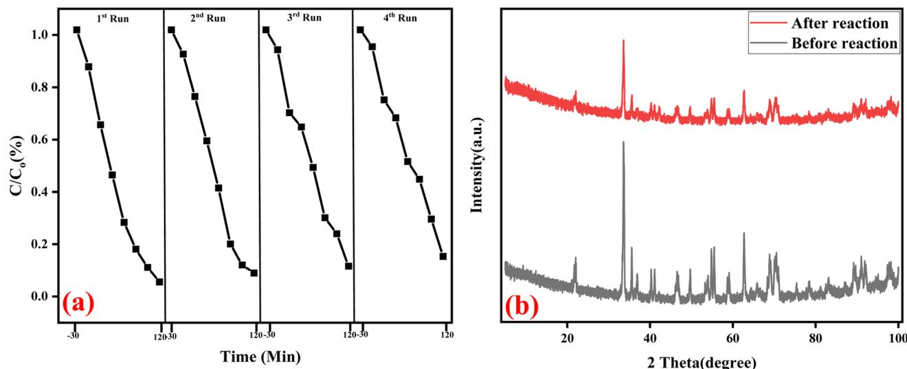
Fig. 12 (a) Successive test run for the degradation of ciprofloxacin and (b) XRD patterns before and after reusing the GO/BiVO<sub>4</sub>/Ag<sub>2</sub>CrO<sub>4</sub> nanocomposites.
