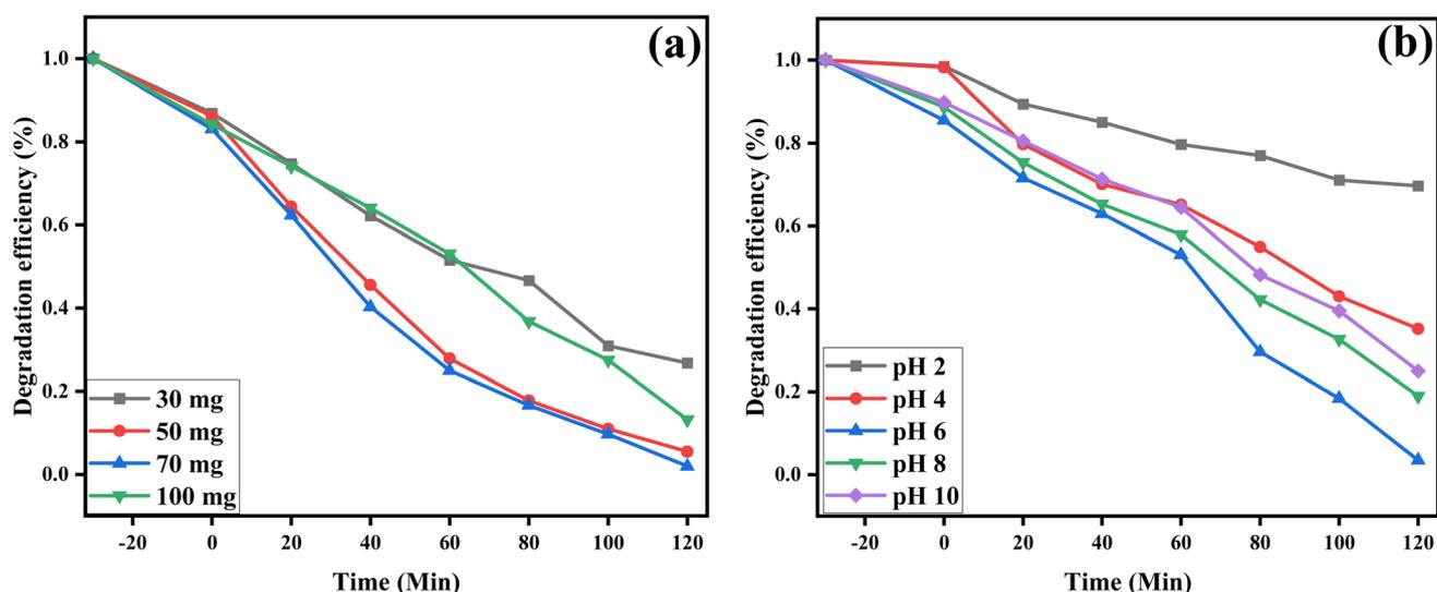
Fig. 11 (a) Effect of dosage plot and (b) pH using the GO/BiVO<sub>4</sub>/Ag<sub>2</sub>CrO<sub>4</sub> nanocomposite.
