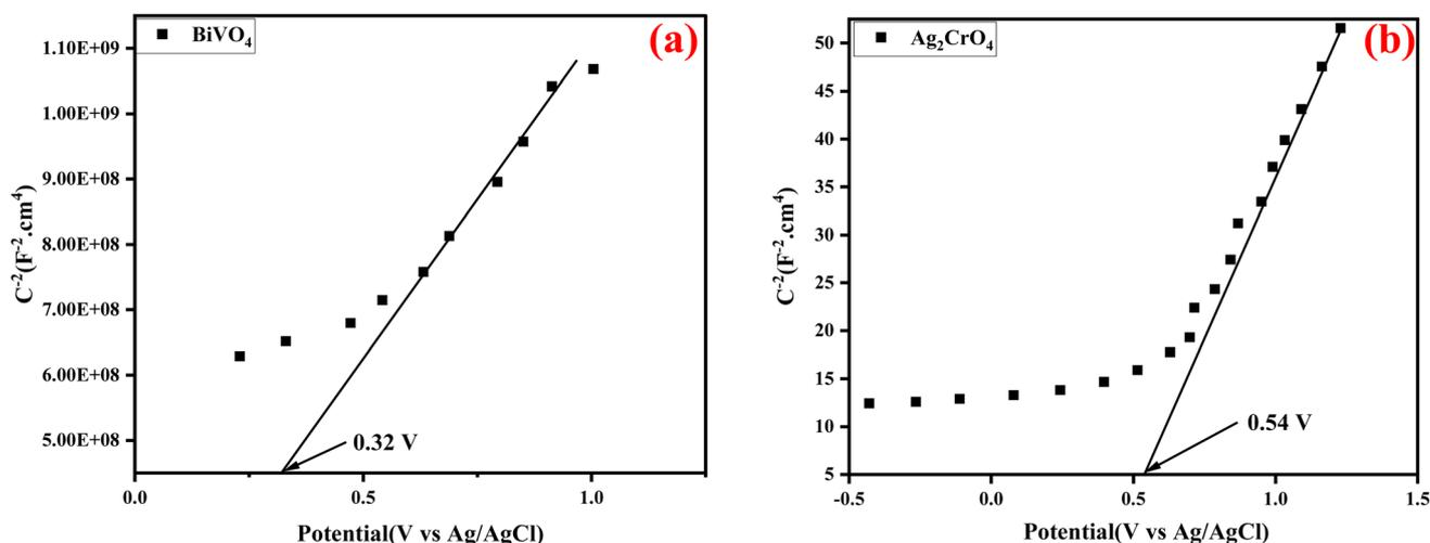
Fig. 14 Mott–Schottky plots of (a) BiVO<sub>4</sub> and (b) Ag<sub>2</sub>CrO<sub>4</sub>.
