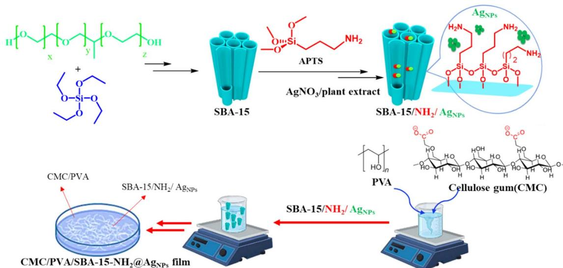
Scheme 2 Schematic illustration of the preparation of the CMC/PVA/SBA-15-NH<sub>2</sub>@AgNPs film.
