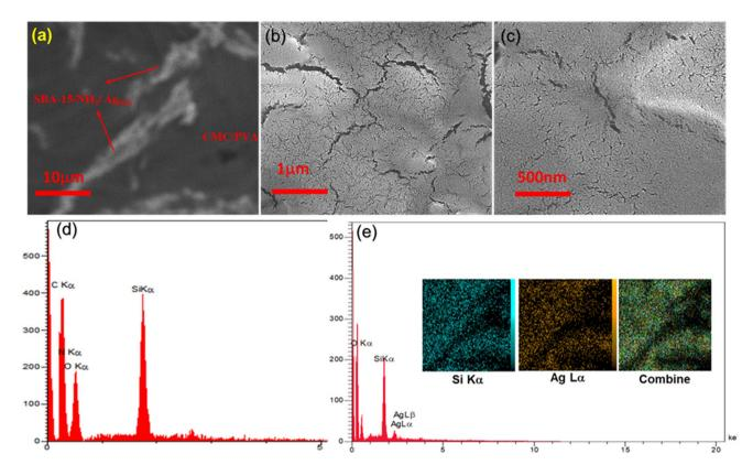
Fig. 2 (a) The HADAF image of the CMC/PVA/SBA-15-NH<sub>2</sub>@AgNPs, (b and c) the SEM images of CMC/PVA/SBA-15-NH<sub>2</sub> and CMC/PVA/SBA-15-NH<sub>2</sub>@AgNPs films, (d and e) EDX analysis of the CMC/PVA/SBA-15-NH<sub>2</sub> and CMC/PVA/SBA-15-NH<sub>2</sub>@AgNPs films, respectively (the inset images are the elemental mapping images of the CMC/PVA/SBA-15-NH<sub>2</sub>@AgNPs film).
