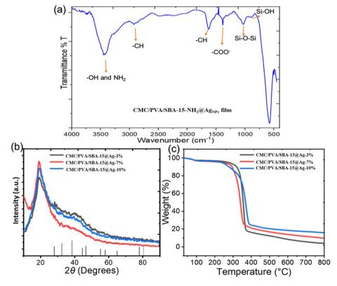
Fig. 1 (a) The FT-IR analysis of the CMC/PVA/SBA-15-NH<sub>2</sub>@AgNPs. (b) XRD patterns of the CMC/PVA/SBA-15-NH<sub>2</sub>@AgNPs films, (c) the TGA plots of the CMC/PVA/SBA-15-NH2@AgNPs films.
