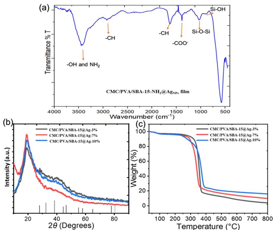
Fig. 1 (a) The FT-IR analysis of the CMC/PVA/SBA-15-NH<sub>2</sub>@AgNPs. (b) XRD patterns of the CMC/PVA/SBA-15-NH<sub>2</sub>@AgNPs films, (c) the TGA plots of the CMC/PVA/SBA-15-NH<sub>2</sub>@AgNPs films.
