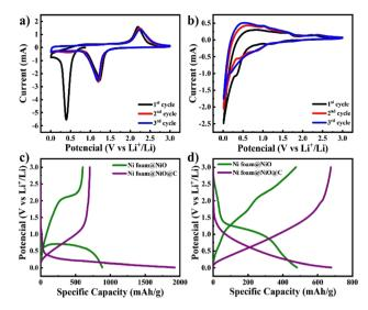
Fig. 5 CV curves of (a) NiO@Ni foam and (b) C@NiO@Ni foam and galvanostatic charge—discharge curves of both electrodes at (c) the 1st cycle and (d) the 100th cycle at current density of 0.1C.
