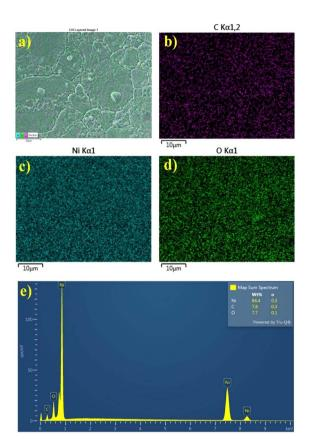
Fig. 4 EDS mapping of C, Ni, and O elements on the (a-d) surface of C@NiO@Ni foam nanostructured branches and (e) EDS spectra.
