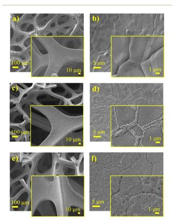
Fig. 3 SEM images of (a and b) Ni foam, (c and d) NiO@Ni foam, and (e and f) C@NiO@Ni foam.
