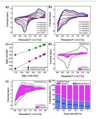
Fig. 8 CV curves of (a) NiO@Ni foam and (b) C@NiO@Ni foam at various scan rates  $(0.1-1 \text{ mV s}^{-1})$ . (c) A logarithmic linear relationship between current and scan rate. Capacitive storage mechanism contribution at a scan rate of 0.9 mV s<sup>-1</sup> for (d) NiO@Ni foam and (e) C@NiO@Ni foam. (f) Capacitive storage contribution at various scan rates for C@NiO@Ni foam.
