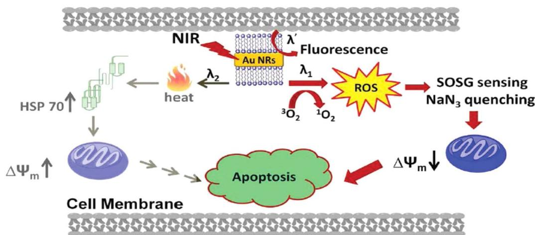
Fig. 8 Various cellular pathways involved in cellular death produced by PDT/PTT effects caused by gold nanorods after photoexcitation (Vankayala *et al.*, 2014).<sup>160</sup>
