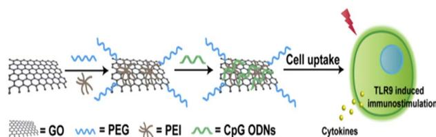
Fig. 27 Schematic depicting the production of GGIC and its immunostimulatory function (Tao *et al.*, 2014).<sup>318</sup>
