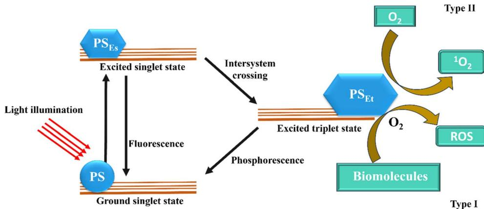
Fig. 2 The PDT's mode of action displays both type I and type II responses. ROS denotes reactive oxygen species, whereas PSEs and PSEt denote PS excited singlet and triplet states (Calixto *et al.* 2016).<sup>42</sup>
