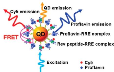
Fig. 10 A single-QD-based nanosensor can detect Rev peptide-RRE association and proflavin inhibitory efficacy using FRET between 605QD and Cy5 (Zhou *et al.* 2005).<sup>182</sup>
