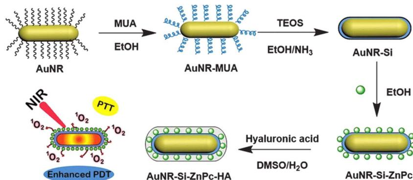
Fig. 28 Schematic representation of AuNR-Si-ZnPc-HA (Tham *et al.*, 2016).<sup>320</sup>
