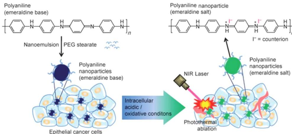
Fig. 22 Scheme for producing naturally occurring photothermal agents using polyaniline nanoparticles and using NIR laser irradiation to kill epithelial cancer cells (Yang *et al.*, 2011).<sup>264</sup>
