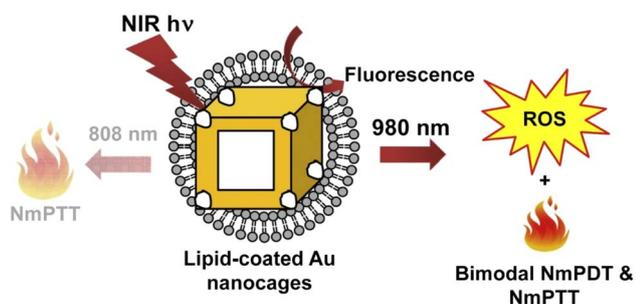
Fig. 20 Photo-induced lipid-coated gold nanocages' working mechanism is illustrated schematically (Vankayala *et al.*, 2014).<sup>240</sup>
