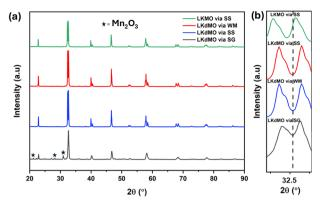
Fig. 2 (a) XRD patterns of the  $LK_dMO$  compounds synthesized *via* SG, WM, and SS and parental compound (LKMO) *via* the SS method, (b) FWHM shift of the  $LK_dMO$  and parental compound (LKMO) samples.
