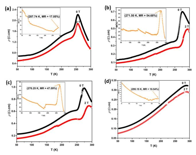
Fig. 14 Resistivity dependence on temperature of  $LK_dMO$  ceramics synthesized by employing (a) SG, (b) WM, (c) SS, and (d) the parental compound through SS under 0 and 2 T. Insets show MR dependence temperature plots for  $LK_dMO$  and LKMO.
