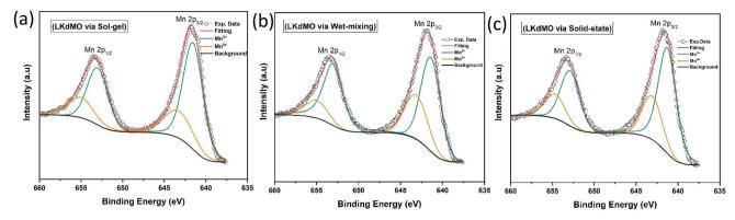
Fig. 10 Narrow scan of Mn 2p XPS spectra of LK<sub>d</sub>MO samples synthesized via (a) the SG, (b) WM, and (c) SS methods.
