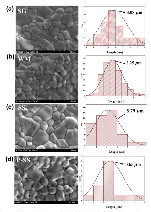
Fig. 5 SEM images of the  $La_{0.85}K_{0.1}\square_{0.05}MnO_3$  compound synthesized *via* (a) SG, (b) WM, and (c) SS, and (d) the parental compound *via* SS.
