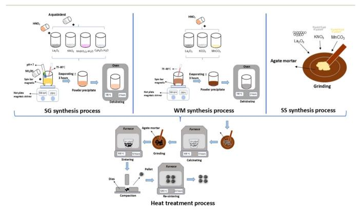
Fig. 1 Process flow of the SG, WM, and SS methods.
