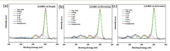
Narrow scan of K 2p and C 1s XPS spectra of LK<sub>rl</sub>MO samples synthesized using (a) the SG, (b) WM, and (c) SS methods.
