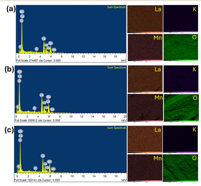
Fig. 6 Elemental mapping image and EDS spectrum of  $LK_dMO$  compounds synthesized by (a) SG, (b) WM, and (c) SS methods
