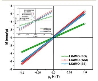
Fig. 12 VSM results of the  $La_{0.85}K_{0.1}\square_{0.05}MnO_3$  compound synthesized using the SG, WM, and SS methods.
