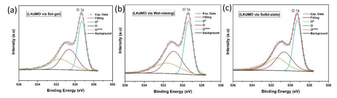
Fig. 11 Narrow scan of O 1s XPS spectra of LK<sub>d</sub>MO samples synthesized via (a) the SG, (b) WM, and (c) SS methods
