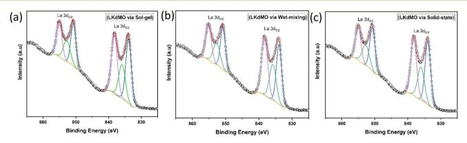
Fig. 8 Narrow scan of La 3d XPS spectra of LK<sub>d</sub>MO samples synthesized using (a) SG, (b) WM, and (c) SS methods.
