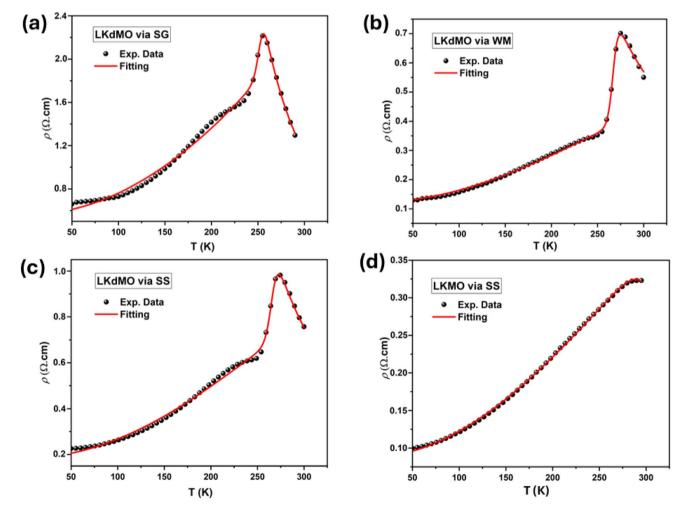
Fig. 16 Fitting curves of  $\rho$ -T data in the entire temperature range of the La<sub>0.85</sub>K<sub>0.1</sub> $\square$ <sub>0.05</sub>MnO<sub>3</sub> samples by (a) SG, (b) WM, and (c) SS and (d) parental compound. Symbols are the experimental results and solid lines are the fitting using eqn (11).
