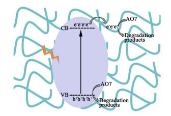
Fig. 7  $\,$  A brief diagram of the AO7 photocatalytic mechanism over MCAP.
