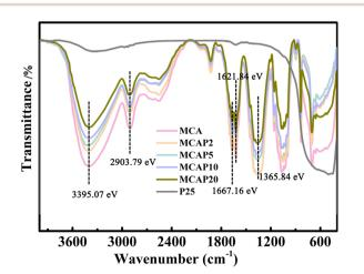
Fig. 2 FT-IR spectra of MCA, MCAP2, MCAP5, MCAP10, MCAP20 and P25.
