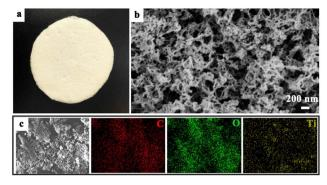
Fig. 1 Photo picture (a), SEM image (b), and mapping images (c) of MCAP20.
