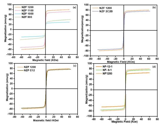
Fig. 3 Hysteresis loop of nickel zinc ferrite (Ni<sub>0.5</sub>Zn<sub>0.5</sub>Fe<sub>2</sub>O<sub>4</sub>) particles.
