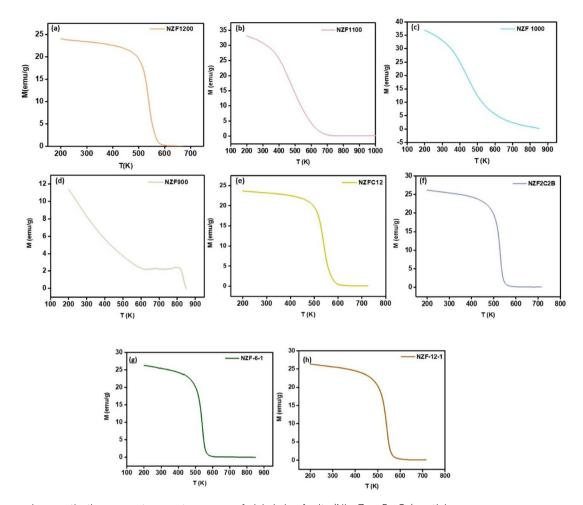
Fig. 5 Measured magnetization versus temperature curve of nickel zinc ferrite (Ni<sub>0.5</sub>Zn<sub>0.5</sub>Fe<sub>2</sub>O<sub>4</sub>) particles.
