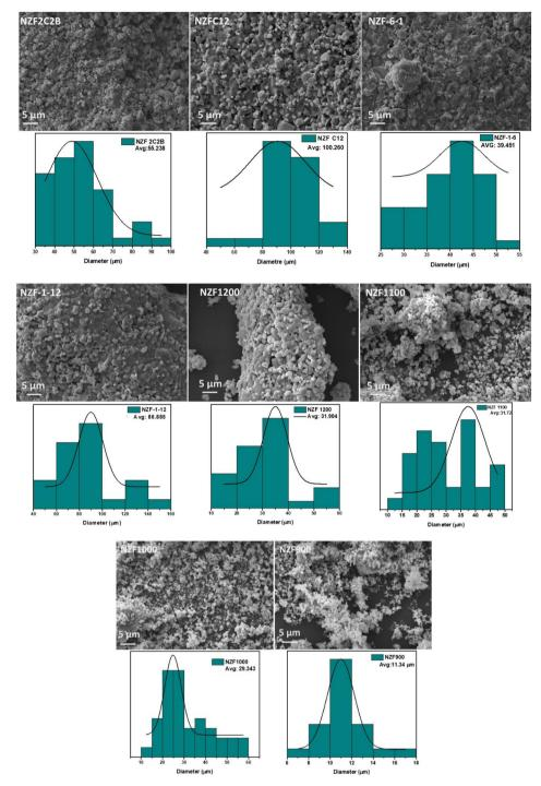
Fig. 2 SEM image and histogram of grain size distribution of all synthesized samples.
