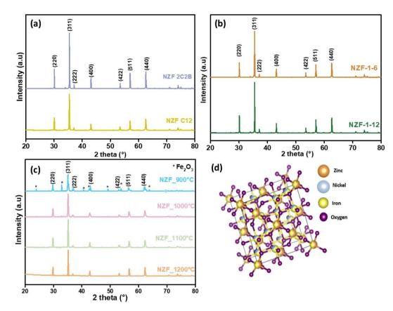
Fig. 1 XRD pattern of nickel zinc ferrite ( $Ni_{0.5}Zn_{0.5}Fe_2O_4$ ) particles. (a) XRD pattern of NZFC12, NZF2C2B. (b) XRD pattern of NZF-1-6, and NZF-1-12. (c) XRD pattern of NZF900, NZF1000, NZF1100, NZF1200. (d) The crystal structure of  $Ni_{0.5}Zn_{0.5}Fe_2O_4$ .
