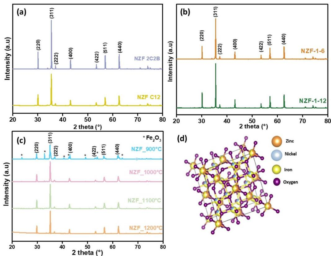
Fig. 1 XRD pattern of nickel zinc ferrite ( $\text{Ni}_{0.5}\text{Zn}_{0.5}\text{Fe}_2\text{O}_4$ ) particles. (a) XRD pattern of NZFC12, NZF2C2B. (b) XRD pattern of NZF-1-6, and NZF-1-12. (c) XRD pattern of NZF900, NZF1000, NZF 1100, NZF1200. (d) The crystal structure of  $\text{Ni}_{0.5}\text{Zn}_{0.5}\text{Fe}_2\text{O}_4$ .
