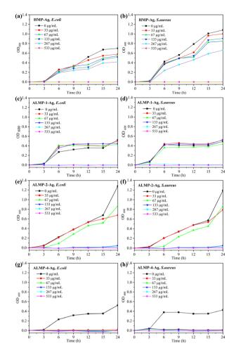
Fig. 5 E. coli and S. aureus growth curves at HMP-Ag (a, b), ALMP-1-Ag (c, d), ALMP-2-Ag (e, f), and ALMP-4-Ag (g, h), respectively.
