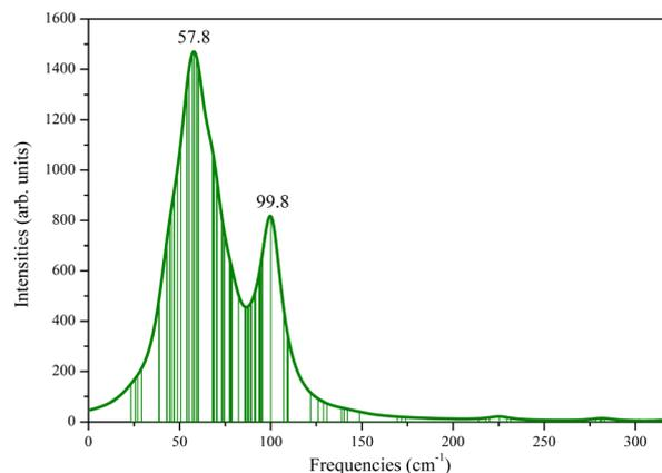
Fig. 2 Simulated Raman spectrum for  $\text{Ag@Mg}_{12}@Ag_{20}$  structure with the Lorentzian smearing of  $20\text{ cm}^{-1}$ , the assumed temperature of 300 K, and the assumed incident light wavelength of 488.00 nm, respectively.
