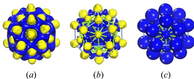
Fig. 4 Electron density for the three-layer Ag@Mg<sub>12</sub>@Ag<sub>20</sub>. Part (a) and part (b) show the deformation electron density with isosurface values of  $0.01 \text{ e } \text{Å}^{-3}$  and  $0.03 \text{ e } \text{Å}^{-3}$  respectively. Part (c) shows the total electron density with isosurface values of  $0.2 \text{ e } \text{Å}^{-3}$ .
