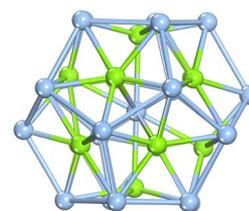
Fig. 1 Configuration of the  $\text{Ag}@\text{Mg}_{12}@\text{Ag}_{20}$  cluster, revealing three concentric structural layers as depicted below. Here, baby blue balls are for Ag atoms and green balls are for Mg atoms, respectively.
