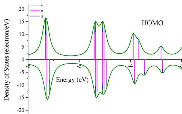
Fig. 5 Partial density of states of the three-layer Ag@Mg<sub>12</sub>@Ag<sub>20</sub> structure. Here, the spin up and spin down states are denoted by the positive and negative DOSs, with the lengths of each vertical line color-coded in pink, blue, and olive to signify the proportion of s, p, and d electrons, respectively. The HOMO level are shown by dashed lines.
