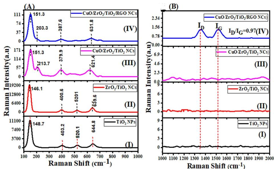
Fig. 6 Raman spectra of pure TiO<sub>2</sub> NPs, ZrO<sub>2</sub>/TiO<sub>2</sub> NCs, CuO/ZrO<sub>2</sub>/TiO<sub>2</sub> NCs, and CuO/ZrO<sub>2</sub>/TiO<sub>2</sub>/RGO NCs.
