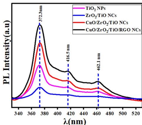
Fig. 8 PL spectra of pure  $\text{TiO}_2$  NPs,  $\text{ZrO}_2/\text{TiO}_2$  NCs,  $\text{CuO}/\text{ZrO}_2/\text{TiO}_2$  NCs, and  $\text{CuO}/\text{ZrO}_2/\text{TiO}_2/\text{RGO}$  NCs.
