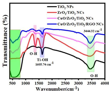
Fig. 7 FT-IR spectra of pure TiO<sub>2</sub> NPs, ZrO<sub>2</sub>/TiO<sub>2</sub> NCs, CuO/ZrO<sub>2</sub>/TiO<sub>2</sub> NCs, and CuO/ZrO<sub>2</sub>/TiO<sub>2</sub>/RGO NCs.
