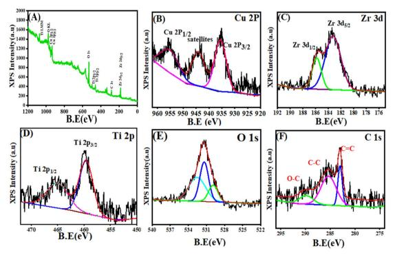
Fig. 5 XPS spectra of CuO/ZrO<sub>2</sub>/TiO<sub>2</sub>/RGO NCs: (A) survey spectra, (B) Cu 2p, (C) Zr 3d, (D) Ti 2p, (E) O 1s, and (F) C 1s.
