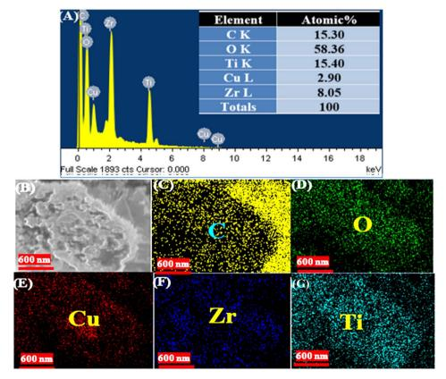
Fig. 4 EDX with elemental mapping of the synthesized CuO/ZrO<sub>2</sub>/TiO<sub>2</sub>/RGO NCs: (A) EDX spectra, (B) electron image, (C) carbon (C), (D) oxygen (O), (E) copper (Cu), (F) zirconium (Zr), and (G) titanium (Ti).
