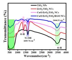
Fig. 7 FT-IR spectra of pure TiO $_2$  NPs, ZrO $_2$ /TiO $_2$  NCs, CuO/ZrO $_2$ /TiO $_2$  NCs, and CuO/ZrO $_2$ /TiO $_2$ /RGO NCs.
