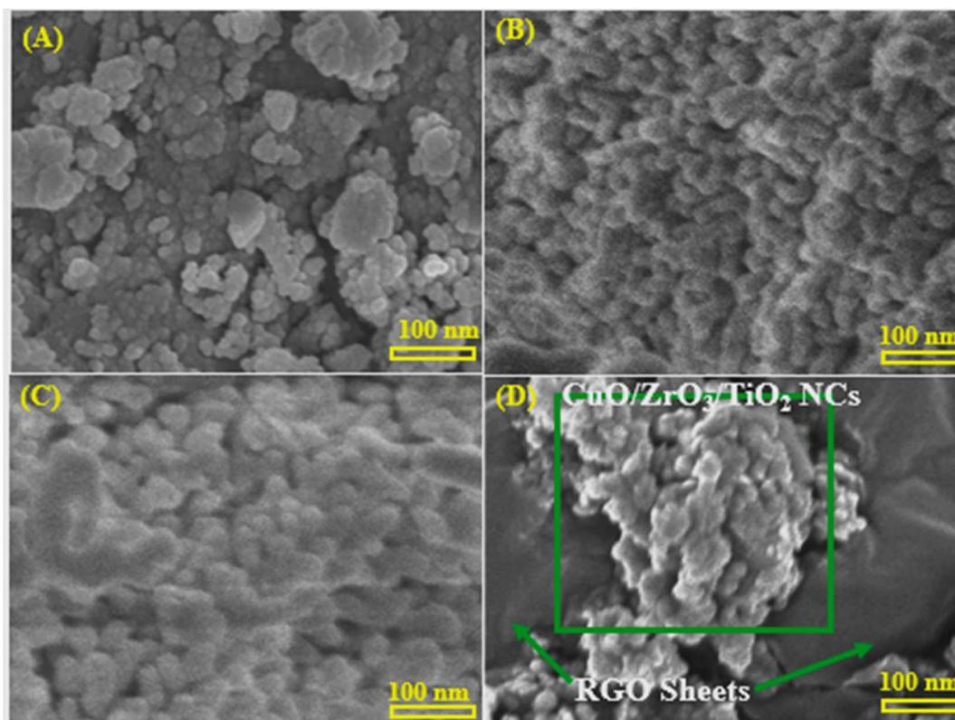
Fig. 3 Scanning electron microscopy (SEM) images: (A) pure  $\text{TiO}_2$  NPs, (B)  $\text{ZrO}_2/\text{TiO}_2$  NCs, (C)  $\text{CuO}/\text{ZrO}_2/\text{TiO}_2$  NCs, and (D)  $\text{CuO}/\text{ZrO}_2/\text{TiO}_2/\text{RGO}$  NCs.
