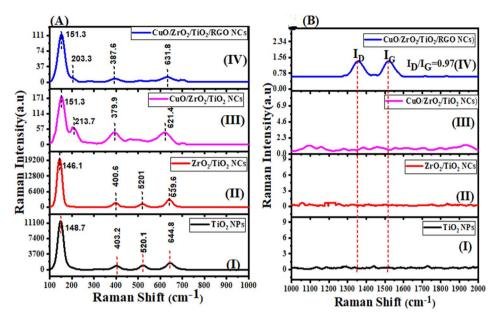
Fig. 6 Raman spectra of pure TiO<sub>2</sub> NPs, ZrO<sub>2</sub>/TiO<sub>2</sub> NCs, CuO/ZrO<sub>2</sub>/TiO<sub>2</sub> NCs, and CuO/ZrO<sub>2</sub>/TiO<sub>2</sub>/RGO NCs.
