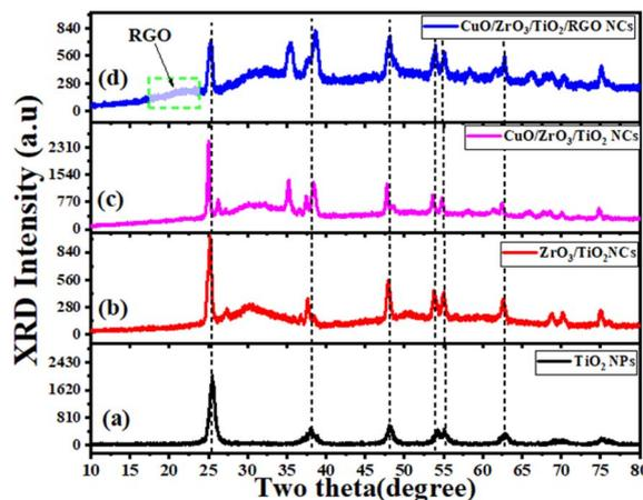
Fig. 1 XRD pattern: (a) pure TiO<sub>2</sub> NPs, (b) ZrO<sub>2</sub>/TiO<sub>2</sub> NPs, (c) CuO/ZrO<sub>2</sub>/TiO<sub>2</sub> NCs, and (d) CuO/ZrO<sub>2</sub>/TiO<sub>2</sub>/RGO NCs.
