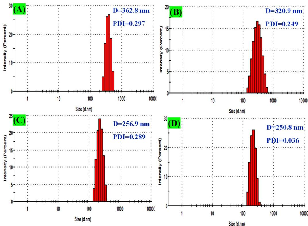
Fig. 9 DLS analysis for particle size distribution: (A) pure  $\text{TiO}_2$  NPs, (B)  $\text{ZrO}_2-\text{TiO}_2$  NCs, (C)  $\text{CuO}-\text{ZrO}_2-\text{TiO}_2$  NCs, and (D)  $\text{CuO}-\text{ZrO}_2-\text{TiO}_2/\text{RGO}$  NCs.
