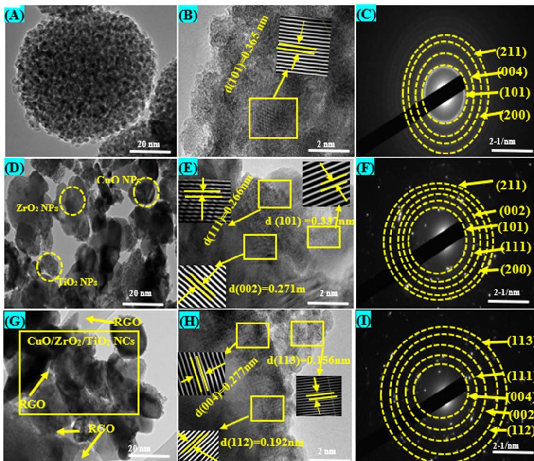
Fig. 2 TEM and HR-TEM images with SAED analysis: (A–C) pure TiO<sub>2</sub> NPs, (D–F) CuO/ZrO<sub>2</sub>/TiO<sub>2</sub> NCs, and (G–I) CuO/ZrO<sub>2</sub>/TiO<sub>2</sub>/RGO NCs.
