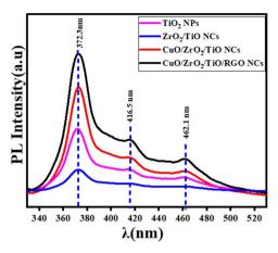
Fig. 8 PL spectra of pure  $TiO_2$  NPs,  $ZrO_2/TiO_2$  NCs,  $CuO/ZrO_2/TiO_2$  NCs, and  $CuO/ZrO_2/TiO_2/RGO$  NCs.
