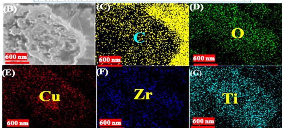
Fig. 4 EDX with elemental mapping of the synthesized  $\text{CuO}/\text{ZrO}_2/\text{TiO}_2/\text{RGO}$  NCs: (A) EDX spectra, (B) electron image, (C) carbon (C), (D) oxygen (O), (E) copper (Cu), (F) zirconium (Zr), and (G) titanium (Ti).
