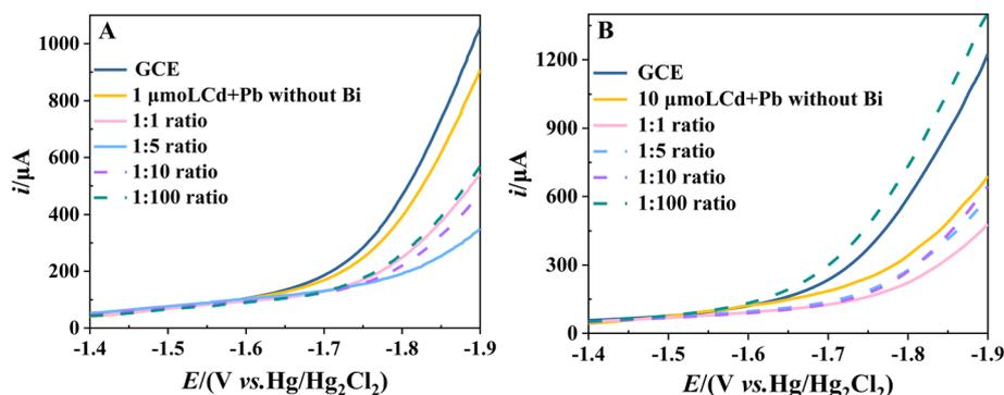
Fig. 7 Cathodic polarization curves of GCE and BiFEs in acetate buffer (pH 4.5). BiFEs are prepared by co-deposition of (A) 1.0  $\mu\text{M}$  and (B) 10  $\mu\text{M}$   $\text{Cd}^{2+} + \text{Pb}^{2+}$  and different excesses of Bi (0, 1, 5, 10 and 100-fold), respectively.
