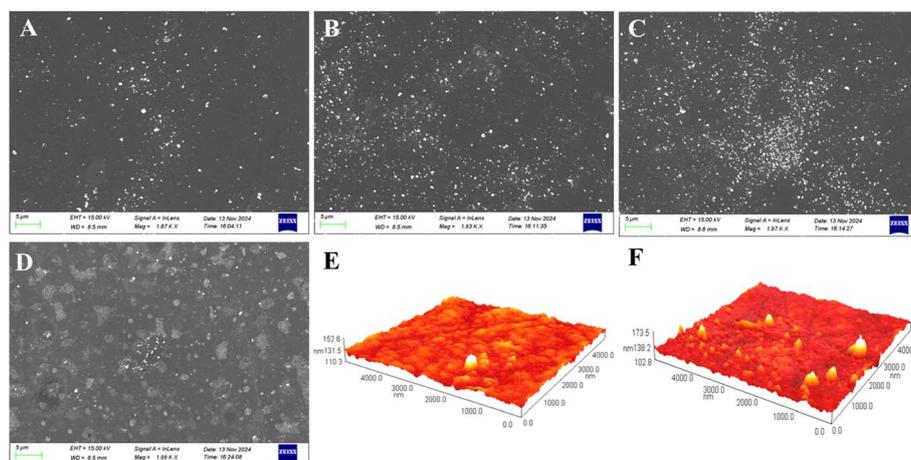
Fig. 4 SEM (A–D) and AFM (E and F) images of different BiFEs. Deposition is carried out from solutions of (A and E)  $0 \mu\text{M}$ , (B)  $10 \mu\text{M}$ , (C and F)  $100 \mu\text{M}$  and (D)  $1000 \mu\text{M Bi(III)}$ , in the presence of  $10 \mu\text{M Cd}^{2+} + \text{Pb}^{2+}$ .
