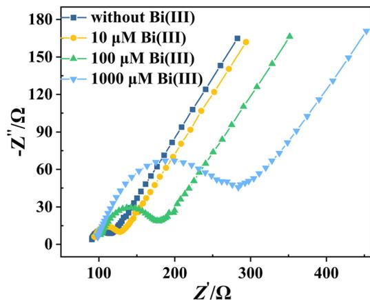
Fig. 3 EIS response of different BiFEs with  $[\text{Fe}(\text{CN})_6]^{3-/4-}$  as the electroactive species. BiFEs are prepared by co-deposition of  $10 \mu\text{M Cd}^{2+} + \text{Pb}^{2+}$  and different concentrations of Bi (0, 10, 100 and  $1000 \mu\text{M}$ , respectively).
