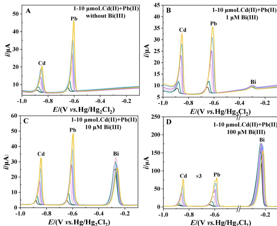
Fig. 1 The stripping voltammograms in the  $\text{Cd}^{2+} + \text{Pb}^{2+}$  solutions at concentrations of  $1, 2, 4, 6, 8$  and  $10$   $\mu\text{M}$  in the presence of (A)  $0$   $\mu\text{M}$  Bi(III), (B)  $1$   $\mu\text{M}$  Bi(III), (C)  $10$   $\mu\text{M}$  Bi(III) and (D)  $100$   $\mu\text{M}$  Bi(III).
