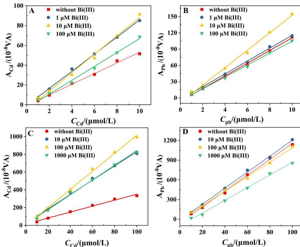
Fig. 2 Calibration curves for (A) Cd and (B) Pb in the presence of 0, 1, 10, and 100  $\mu M$  Bi over the 1–10  $\mu M$  concentration range, and (C) Cd and (D) Pb in the presence of 0, 10, 100, and 1000  $\mu M$  Bi over the 10–100  $\mu M$  concentration range.
