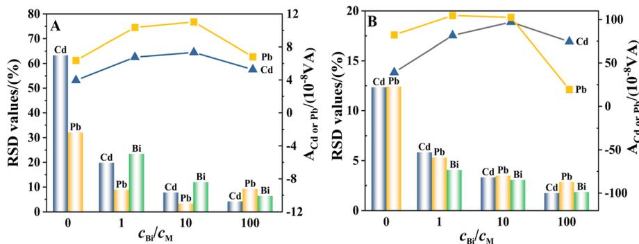
Fig. 5 The RSD values of the peak areas of Cd, Pb and Bi and the peak areas of Cd and Pb at different  $c_{Bi}/c_M$  ratios. In the DPASV measurements, the concentrations of Cd and Pb are constant and the same, 1  $\mu M$  (A) and 10  $\mu M$  (B), respectively, while the concentrations of Bi are 0, 1, 10 and 100 times higher than those of Cd and Pb, respectively.
